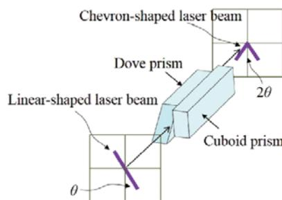
Fig. 1 Formation of a chevron-shaped laser beam from a linear-shaped beam passing through a one-sided dove prism with a tilt angle  $\theta$  from the junction plane of the prism [1].
