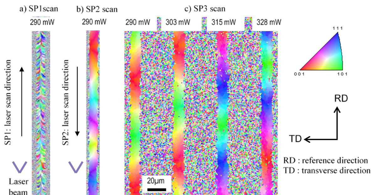
Fig. 2 EBSD orientation map showing (a) lateral growth of polycrystals after a single 290-mW laser scan following the pattern SP1; (b) single-grain growth after a single 290-mW laser scan following the pattern SP2; (c) double laser scan following the pattern SP3, with variation of laser power. The crystals are colored following the inset triangle color code, which corresponds to the alignment of the crystal directions with the surface normal of the Al film.
