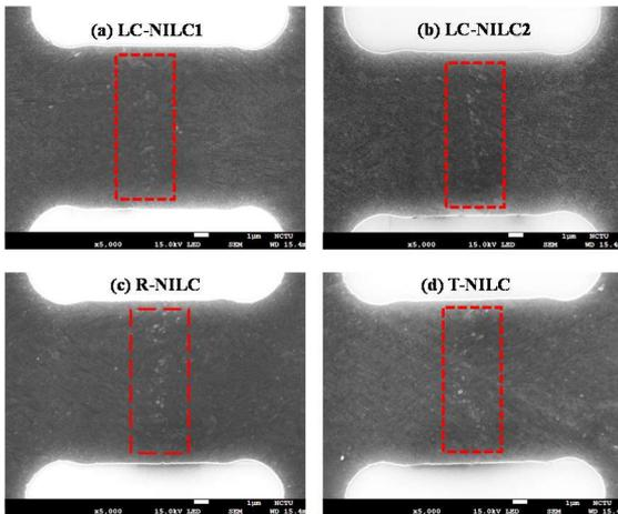
Fig. 4. SEM images of the channel region for (a)-(c) NILC poly-Si thin film with different preheating temperatures and (d) T-NILC.
