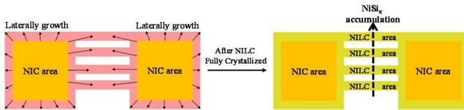
Fig. 3. Schematic of NiSi<sub>x</sub> accumulation in the channel region.
