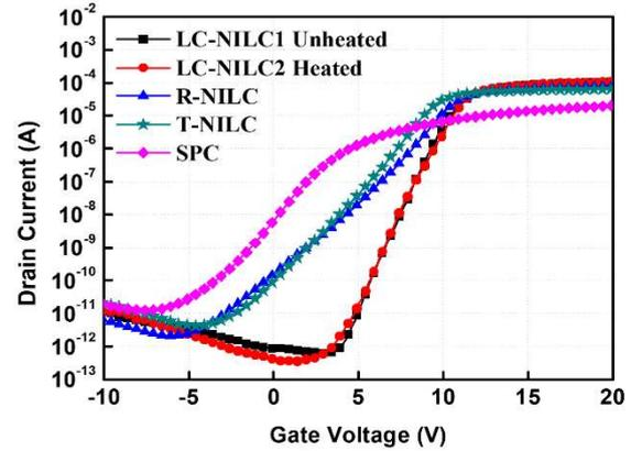
Fig. 5. Comparison of I<sub>D</sub>-V<sub>G</sub> transfer curves in LC-NILC1~2 to R-NILC, T-NILC, and SPC poly-Si TFTs.
