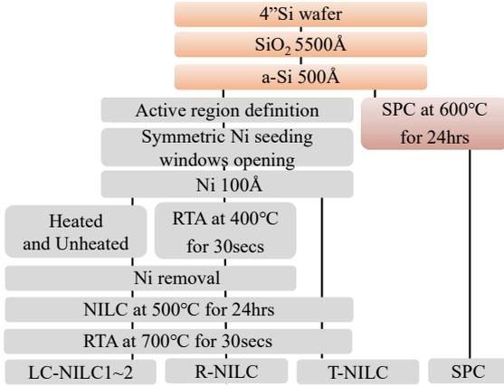
Fig. 2. Process flows for symmetric NILC and SPC poly-Si TFTs
