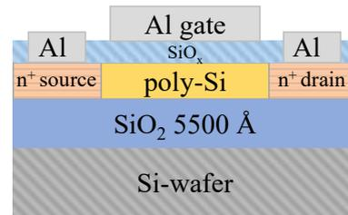
Fig. 1. Schematic of LC-NILC poly-Si TFTs cross-section.
