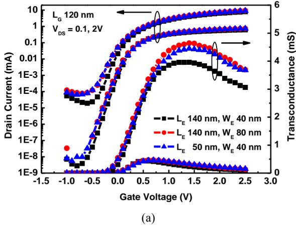
Fig. 2 (a) Transfer and (b) output characteristics of trigate TFTs with different S/D extension lengths and widths. The gate length and unit channel width are 120 nm and 40 nm, respectively.
