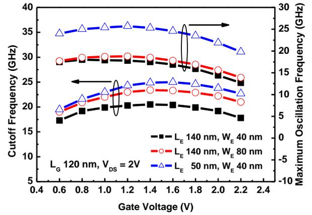
Fig. 3 Cutoff frequency and maximum oscillation frequency of trigate TFTs with different extension lengths and widths. The gate length and unit channel width are 120 nm and 40 nm, respectively.
