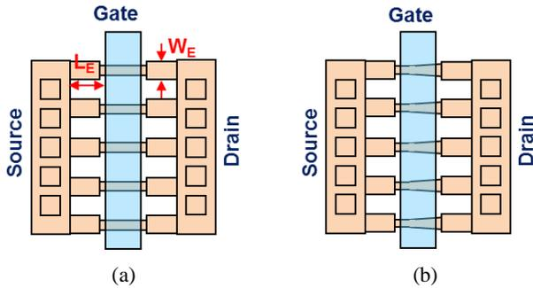
Fig. 1 Layout structure of multi-channel trigate TFTs in a unit cell with (a) standard and (b) tapered channel structures.
