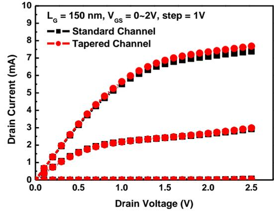
Fig. 4 Output characteristics of trigate TFTs with different channel layout designs. The gate length and unit average channel width are 150 nm and 50 nm, respectively.
