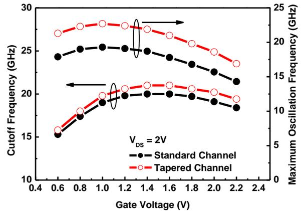
Fig. 5 Cutoff frequency and maximum oscillation frequency of trigate TFTs with different channel layout designs. The gate length and unit average channel width are 150 nm and 50 nm, respectively.
