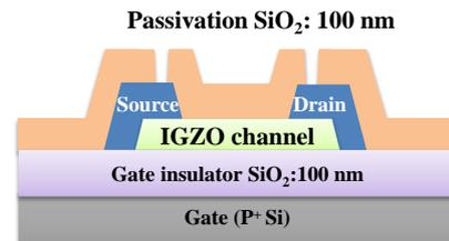
Fig. 1 Schematic cross-sectional view of the TFT.
