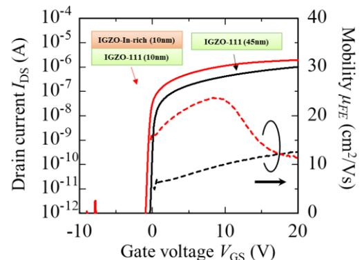
Fig. 2 Transfer characteristics of the IGZO111 and IGZO-In-rich/111 hetero-channel TFTs ( $V_{DS}=0.1$  V). Solid and dotted lines represent a drain current and a field effect mobility, respectively.
