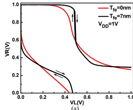
Fig. 8. (a) At  $V_{DD} = 1\text{V}$ , NC-FinFET SRAM cell with  $T_{fe} = 7\text{nm}$  shows smaller WSNM and larger  $V_{write,0}$  than FinFET SRAM cell. (b) NC-FinFETs exhibit larger drain saturation voltage [ $V_{dsat} = (V_G - V_t)/m$ ], and both pull-up and pass-gate devices operate in the linear region which increases the  $V_{write,0}$  and decreases WSNM. Negligible hysteresis window of WSNM is observed for NC-FinFET SRAM cell.
