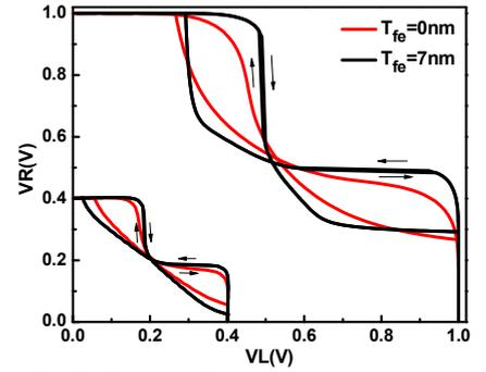
Fig. 3. The butterfly curves for determining the RSNM of NC-FinFET and FinFET SRAM cells in the near-/sub-threshold ( $V_{DD} = 0.4\text{V}$ ) and superthreshold ( $V_{DD} = 1\text{V}$ ) regions. NC-FinFETs show better RSNM. Negligible hysteresis window of RSNM is observed for NC-FinFETs SRAM cell at  $V_{DD} = 1\text{V}$  and  $0.4\text{V}$ .
