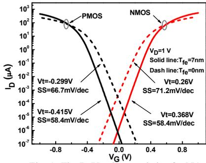
Fig. 1. The  $I_D$ - $V_G$  characteristics for NC-FinFETs ( $T_{fe} = 7\text{nm}$ ) and FinFETs ( $T_{fe} = 0\text{nm}$ ) at  $V_D = 1\text{V}$ . NC-FinFETs show larger threshold voltage and better subthreshold swing than FinFETs.
