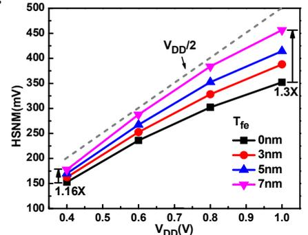
Fig. 9. The hold static noise margin (HSNM) for 6T FinFET ( $T_{fe} = 0\text{nm}$ ) and NC-FinFET ( $T_{fe} = 3\text{nm} \sim 7\text{nm}$ ) SRAM cells in the near-/subthreshold and superthreshold regions. When  $T_{fe} = 7\text{nm}$ , it shows superior HSNM and nearly close to the  $V_{DD}/2$  line.
