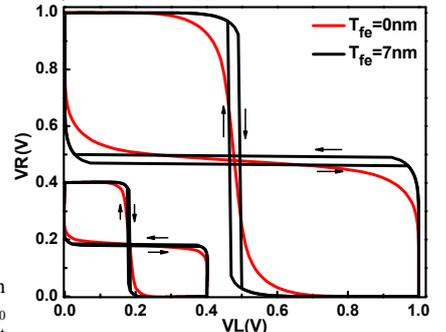
Fig. 10. The butterfly curves of HSNM for NC-FinFET and FinFET SRAM cells in the subthreshold and superthreshold regions. NC-FinFETs SRAM shows better HSNM at  $V_{DD} = 1\text{V}$  and  $0.4\text{V}$ . At  $V_{DD} = 1\text{V}$ , hysteresis is observed for HSNM.
