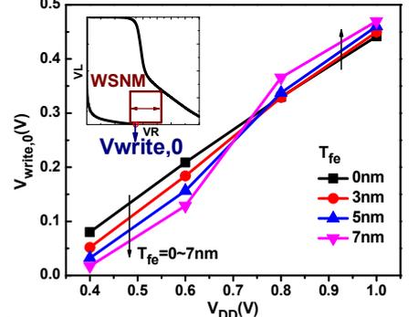
Fig. 6. NC-FinFETs SRAM cell with  $T_{fe} = 7\text{nm}$  exhibits larger  $V_{write,0}$  at  $V_{DD} = 1\text{V}$  but smaller  $V_{write,0}$  at  $V_{DD} = 0.4\text{V} \sim 0.6\text{V}$ . The inset shows the definitions of WSNM and  $V_{write,0}$ . For SRAM cell, WSNM increases as  $V_{write,0}$  decreases.
