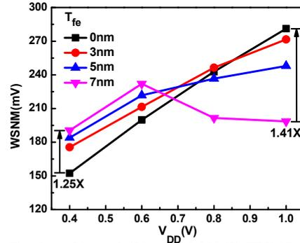
Fig. 5. At  $V_{DD} = 0.4\text{V} \sim 0.6\text{V}$ , NC-FinFET SRAM cells ( $T_{fe} = 3\text{nm} \sim 7\text{nm}$ ) show larger write static noise margin (WSNM) than the FinFET SRAM cell ( $T_{fe} = 0\text{nm}$ ). At  $V_{DD} = 1\text{V}$ , NC-FinFET SRAM cells show lower WSNM than the FinFET SRAM cell, while NC-FinFET SRAM cell with  $T_{fe} = 7\text{nm}$  still exhibits adequate WSNM ( $= 198\text{mV}$ )
