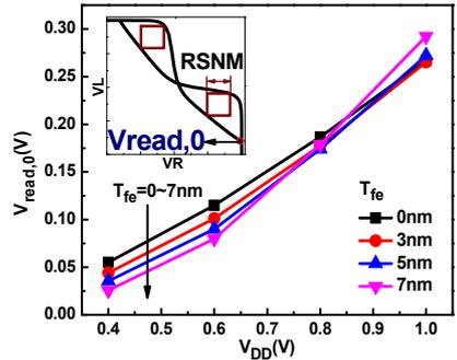
Fig. 4. At  $V_{DD} = 0.4\text{V} \sim 0.6\text{V}$  (near-/subthreshold region), NC-FinFET SRAM cell shows lower read disturb voltage ( $V_{read,0}$ ) than the FinFET SRAM cell due to improved subthreshold swing. The inset shows the definitions of RSNM and  $V_{read,0}$ . RSNM increases as  $V_{read,0}$  decreases.
