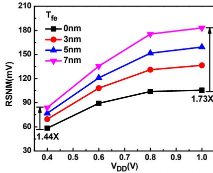
Fig. 2. The read static noise margin (RSNM) for 6T FinFET ( $T_{fe} = 0\text{nm}$ ) and NC-FinFET ( $T_{fe} = 3\text{nm} \sim 7\text{nm}$ ) SRAM cells in the near-/sub-threshold and superthreshold regions. NC-FinFET ( $T_{fe} = 7\text{nm}$ ) SRAM cell exhibits 1.73 times (1.44 times) larger RSNM than FinFET SRAM cell at  $V_{DD} = 1\text{V}$  ( $V_{DD} = 0.4\text{V}$ ). As  $T_{fe}$  increases, RSNM of NC-FinFET SRAM cell increases.
