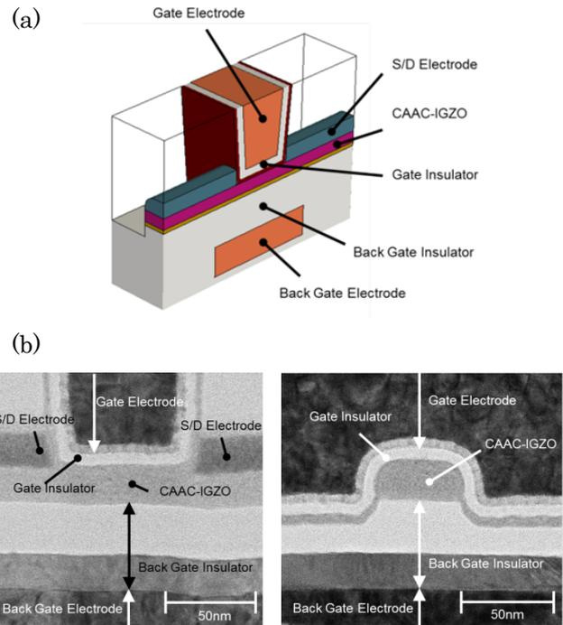
Fig.1 (a) Schematic diagram of TGSA structure and (b) Cross-sectional STEM images (left: L-direction, right: W-direction).
