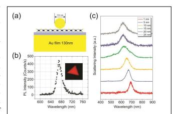
**Figure 1. NGMF nanostructure schematic and characterization.** (a) Illustration of MoS<sub>2</sub> monolayer situated into a NGMF system with various gap thickness. (b) Typical PL spectrum of MoS<sub>2</sub> monolayer on glass substrate. Inset: PL intensity mapping a MoS<sub>2</sub> monolayer sample. (c) Dark field scattering spectrum of NGMF systems with various gap thicknesses.
