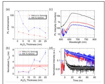
**Figure 2. Spontaneous emission modification of MoS2 monolayer coupled to NGMF.** (a-b): MoS2 monolayer PL intensity enhancement (a) and fast decay (b) as a function of spacer thicknesses. (c-d): Typical PL spectra (c) and decay curves (d) of MoS2 monolayer coupled to NGMF. The black, red, and blue curves correspond to the 1, 15, and 25 nm spacer, respectively.
