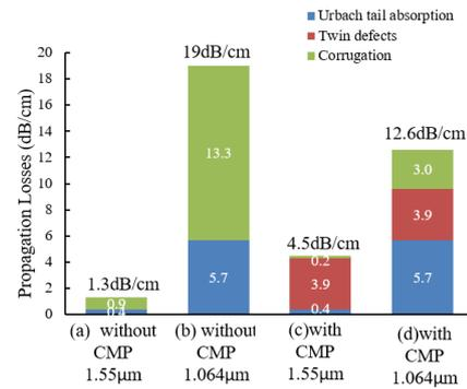
Fig. 5 Bar charts of propagation losses of the waveguides fabricated without CMP process (a)(b) and with CPM process (c)(d). (a) and (c) are measured at 1.55 μm (TE polarization), and (b) and (d) are measured at 1.064 μm (TM polarization).
