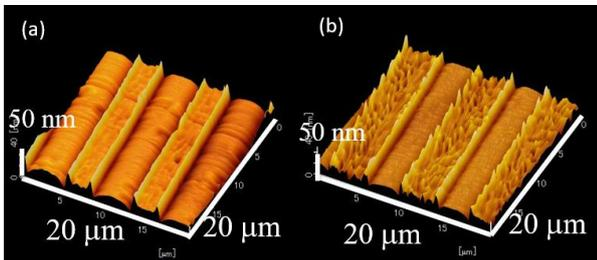
Fig. 2 Surface AFM images of the waveguides fabricated without CMP process (a) and with CMP process (b).
