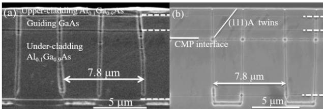
Fig. 1 Cross-sectional SEM images of the waveguides fabricated without CMP process (a) and with CMP process (b).
