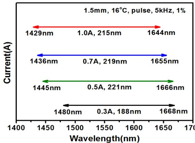
Fig. 4 Tuning range limits of the QD-EC laser, obtained under different injection currents.
