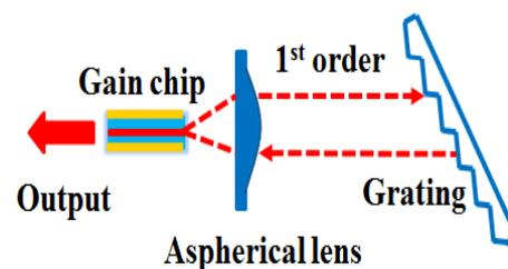
Fig. 2 Sketch of external cavity laser in Littrow configuration.
