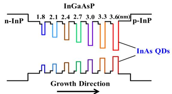
Fig. 1 Schematic energy diagram of the epitaxial layer structure for the chirped QD laser.
