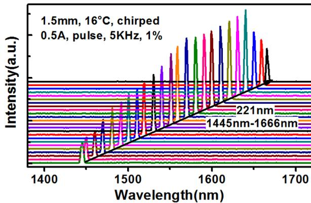
Fig. 3 Tuning spectra of the QD-EC laser, obtained under a pulsed injection current of 0.5A.
