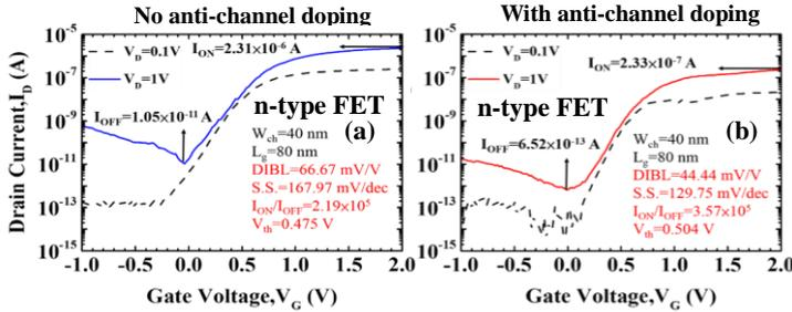
**Fig.3**  $I_{DS}$ - $V_{GS}$  curves of n-type JAM-FETs (a) without anti-channel doping, and (b) with anti-channel doping for the device dimension of  $W/L = 40/80$  nm. The  $I_{ON}/I_{OFF}$  ratio is calculated by the  $I_{DS}$ - $V_{GS}$  curve at  $V_{DS}=1.0V$
