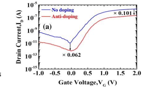
**Fig.7** (a)  $I_{DS}$ - $V_{GS}$  and (b)  $I_{DS}$ - $V_{DS}$  characteristics of n-type JAM-FET with and without anti-channel doping for the device dimension of  $W/L = 40/80$  nm.
