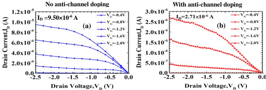
**Fig.6**  $I_{DS}$ - $V_{DS}$  characteristics of p-type JAM-FET (a) without and (b) with anti-channel doping for the device dimension of  $W/L = 40/80$  nm.
