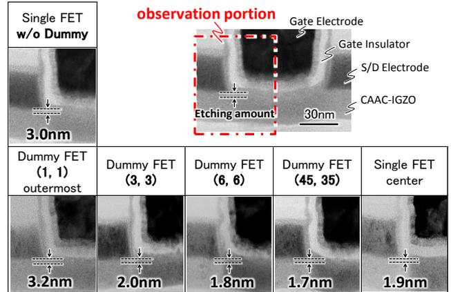
Fig. 3 Cross-sectional STEM image of FET used for loading effect examination.
