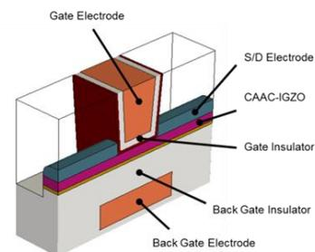
Fig. 1 Trench-gate self-aligned structure.
