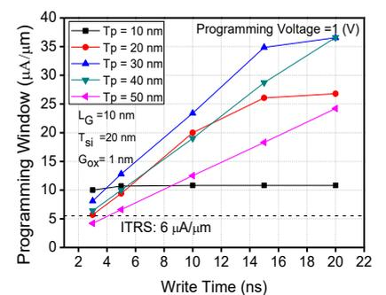
Fig. 9. Programming window versus write time under different  $T_p$ .
