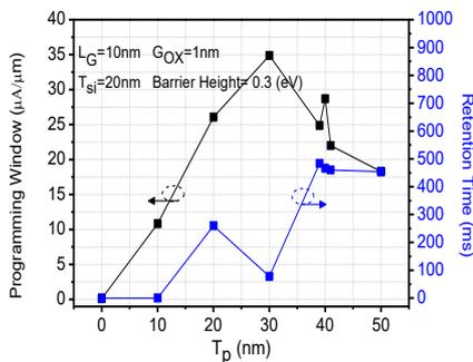
Fig. 4. The programming window and retention time versus the variation of  $T_p$  at 300K. The better performance is derived as  $T_p = 40$ nm.
