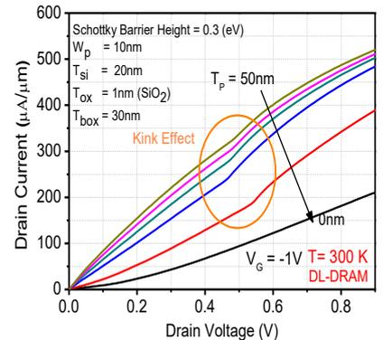
Fig. 3.  $I_D$ - $V_D$  Characteristics of different thickness of body. It can be clearly seen that kink effect occurs on the curve.
