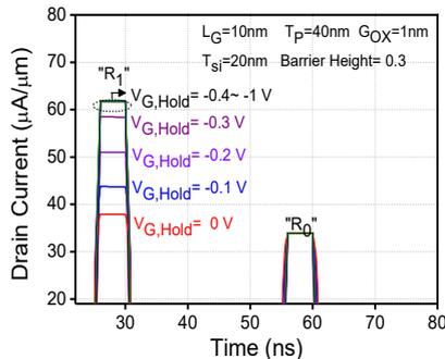
Fig. 5. Drain currents and programming window versus different hold biases.
