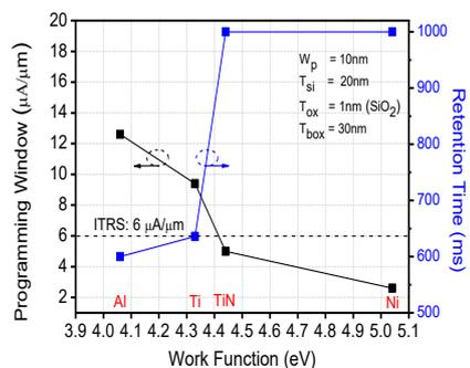
Fig. 7. Programming window and retention time of different Metal materials of source and drain contacts.
