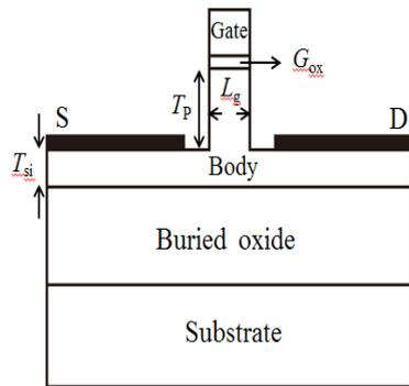
Fig. 1. The structure of Doping-less 1T-DRAM with suitable work function material for source and drain electrodes. The hole can store in the raised body.
