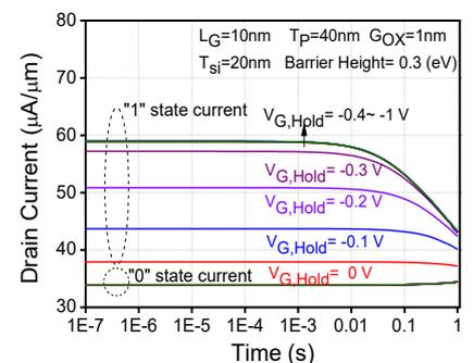
Fig. 6. Retention time versus different hold biases.
