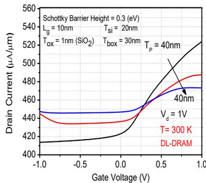
Fig. 2.  $I_D$ - $V_G$  Characteristics for different  $T_p$ . We demonstrate that  $T_p$  will influence gate controllability.
