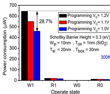
Fig. 8. Power consumption of different DRAM operating state for different drain bias.
