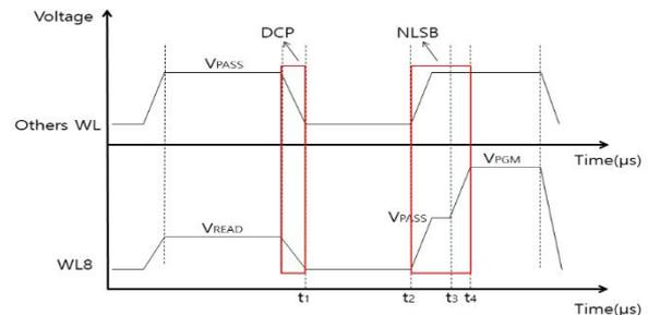
Fig. 2 The timing Diagram of DCP and NLSB
