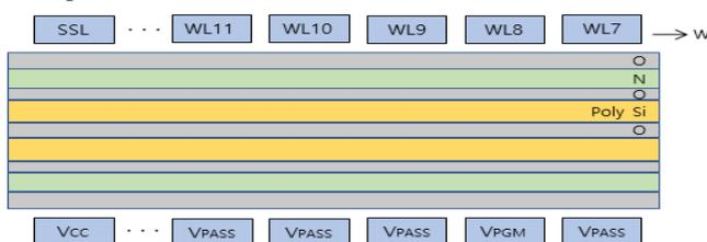
Fig. 1 Simplified vertical diagram of 3D NAND flash
