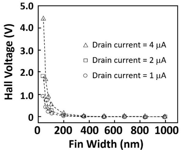
Fig. 4. The output Hall voltage at different drain current and fin width at  $B = 0.1T$ . The Hall voltage is enhanced when the fin width is reduced below 100nm.
