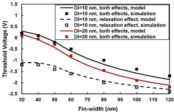
Fig. 2. Verification of the threshold voltage model with TCAD simulation at different values of fin width and dielectric thickness.
