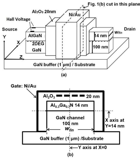
Fig. 1. (a) 3D schematic of the MIS-FinFET structure with Hall sensor; (b) X-Y cross-sectional schematic of the structure.
