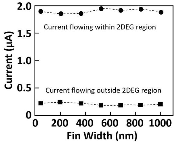
Fig. 3. Current distribution in the fin region between that flowing within the 2DEG region and that flowing outside the 2DEG region in the GaN.
