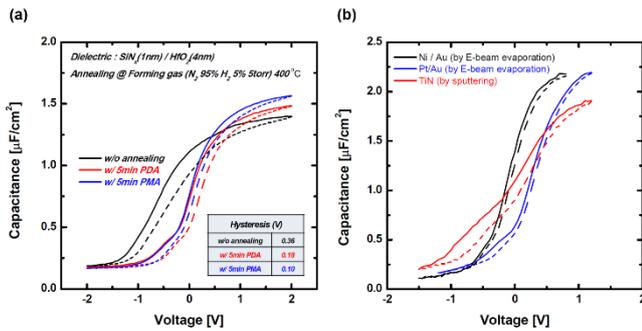
Fig. 2 C- $V_G$  characteristics for (a) different annealing conditions, and (b) different gate metals
