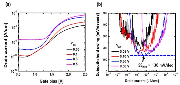
Fig. 3 (a)  $I_D$ - $V_G$  characteristics, and (b) Extracted SS of fabricated  $\text{In}_{0.53}\text{Ga}_{0.47}\text{As}$  homo-junction TFET
