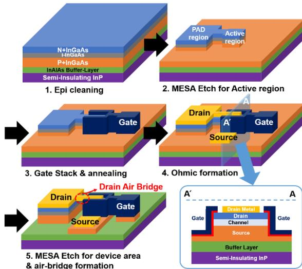
Fig. 1 Process flow and cross-sectional view of  $\text{In}_{0.53}\text{Ga}_{0.47}\text{As}$  homo-junction TFET.
