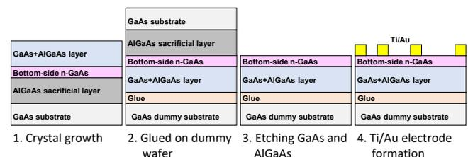
Fig. 2 Schematic illustration of the process after growth.
