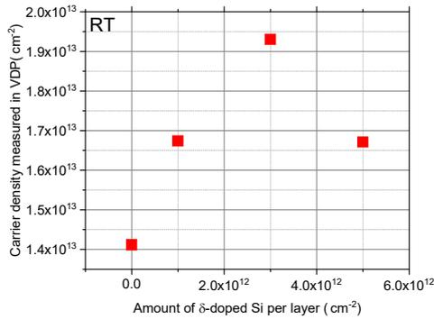
Fig. 3 Carrier density depending on the amount of  $\delta$ -doped Si.
