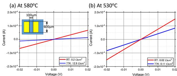
Fig. 4 I-V curves between two electrodes. The upper layers were grown at (a)  $580^\circ\text{C}$  and (b)  $530^\circ\text{C}$ . The inset of (a) shows the measurement configuration.
