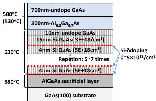
Fig. 1 Schematic illustration of the sample structure.
