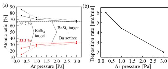
Fig. 1. (a) Ba and Si atomic ratios against  $P$  for samples sputtered without (dotted lines) and with (solid lines) the presence of Ba source on the BaSi<sub>2</sub> target, and (b) dependence of measured deposition rate of the sputtered film decreased on  $P$  by presence of the Ba source on the BaSi<sub>2</sub> target (solid lines).
