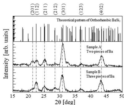
Fig. 2. GI-XRD patterns of the films sputtered at 600 °C on a Si(111) substrate by adding two or three Ba sources on the BaSi<sub>2</sub> target.
