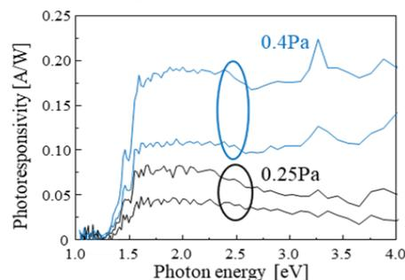
Fig. 4. Photoresponse spectra of sample B after the a-Si cap under various bias voltages.
