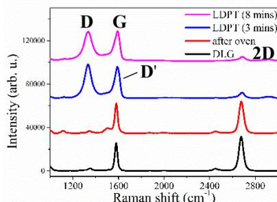
Fig. 1. Raman spectra of the DLGs before and after LDPT.
