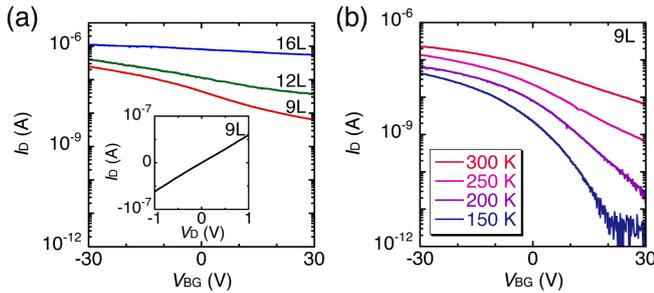
**Fig. 3** (a)  $I_D$ - $V_{BG}$  plots with the different number of layers at RT and  $V_D = 1$  V. (b)  $I_D$ - $V_{BG}$  plots of 9L in 300–150 K at  $V_D = 1$  V.
