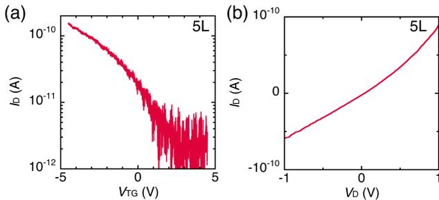
**Fig. 4** (a)  $I_D$ - $V_{TG}$  plot at  $V_D = 1$  V and (b)  $I_D$ - $V_D$  plot at  $V_{TG} = 0$  V of 5L SnS at RT.
