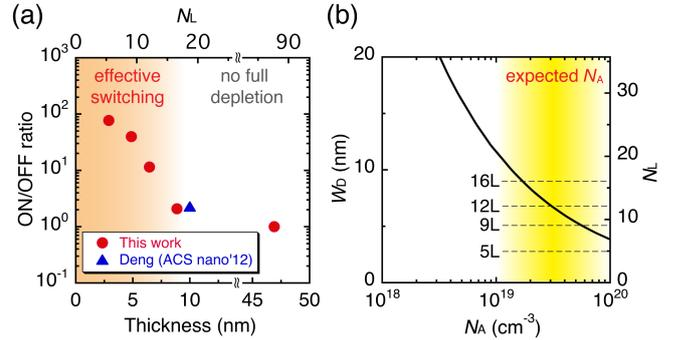
**Fig. 5** (a) Current modulation  $I_{ON}/I_{OFF}$  versus thickness. (b) Relationship between depletion width  $W_D$  and acceptor density  $N_A$ .
