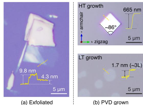
Fig. 1 Typical optical images of SnS via (a) Au-exfoliation and (b) PVD. Insets: AFM height profiles along the dashed lines.
