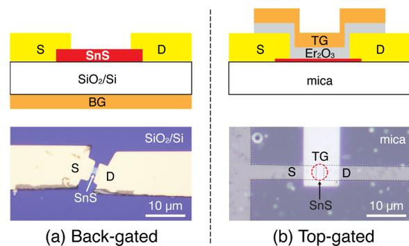
Fig. 2 Cross-sectional illustration and optical image of (a) back-gated and (b) top-gated FET.
