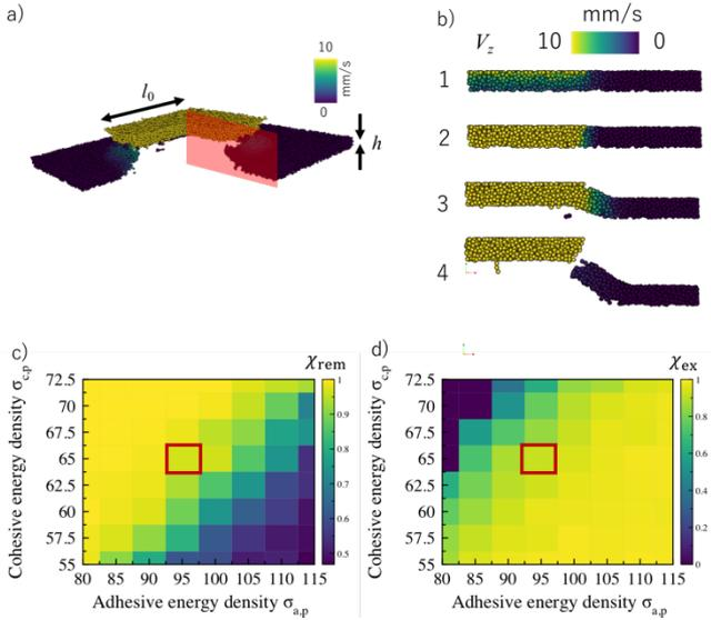
Fig.2 (a) A snapshot and (b) cross-sections of ROP patterning simulation by DEM. (c-d) Colormaps on patterning quality indicators  $\chi_{rem}$  and  $\chi_{ex}$  as functions of particle interactions  $\sigma_{c,p}$  and  $\sigma_{a,p}$ . The condition shown in (a-b) is indicated by the red boxes.
