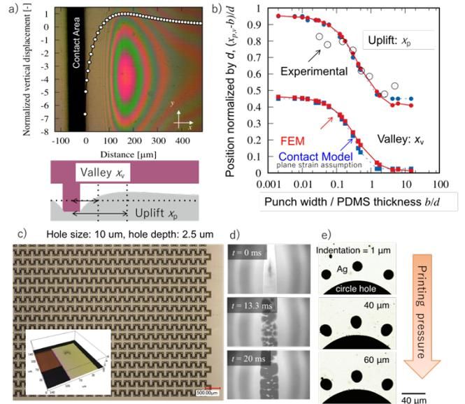
Fig.3 (a) Direct observation of PDMS deformation upon contact with a flat bar punch together with a predicted deformation profile. (b) PDMS pile-up phenomena. (c) Vertical interconnection enabled by the deformation of PDMS. (d) initial contact dynamics of PDMS blanket on a glass substrate. (e) pattern fidelity worsening phenomena originated from horizontal PDMS deformation.
