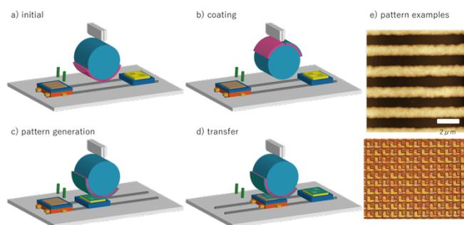
Fig.1 A schematic of reverse offset printing: (a) initial, (b) coating (c) pattern generation (off step) and (d) transfer (set step). (e) Pattern examples of (top) a L/S 1  $\mu\text{m}$  silver pattern and (bottom) a TFT array.
