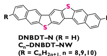
Fig. 2 Chemical structures of DNBDT-N derivatives.
