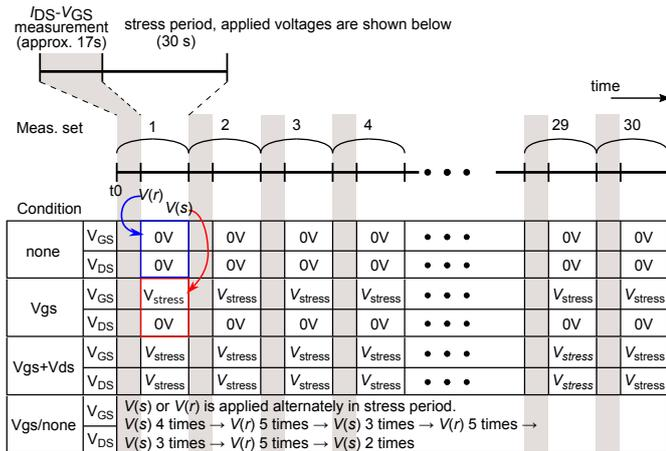
Fig. 3: Measurement sequences for four stress conditions. A set of I-V curve measurement and stress application, which take approximately 17s and 30s, are repeated for 30 times. “Vgs/none” apply “Vgs” stress condition ( $V(s)$ ;  $V_{GS} = V_{stress}$ ,  $V_{DS} = 0.0V$ ) and “none” condition ( $V(r)$ ;  $V_{GS} = V_{DS} = 0.0V$ ) alternatively.
