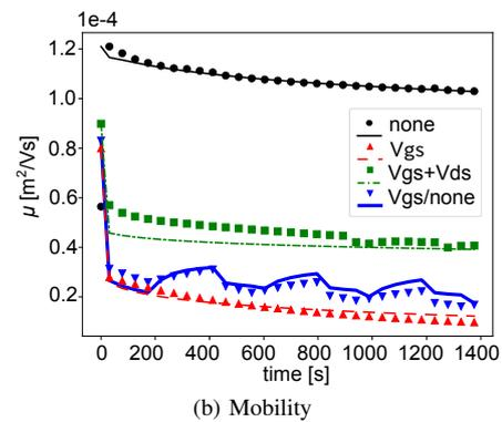
Fig. 6: Extracted threshold voltages and carrier mobility during the measurement of Fig. 5-(b) are shown as symbols. The fitting results using the proposed model are also plotted with lines.
