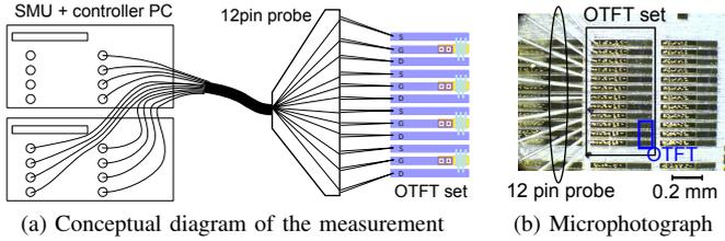
Fig. 2: Parallel Kervin measurement of four OTFTs in a OTFT set. Bias voltage application and current measurements are automated by controller PC. (a) Each terminal is independently controlled by respective SMU channel. (b) The OTFT set under probing.
