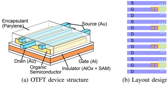
Fig. 1: Transistor structure and the layout of a OTFT set. Four independent OTFTs in an OTFT set are measured in a parallel manner using a 12-pin DC probe. Probing pads of the OTFT set are drawn long to improve endurance against repetitive probing.
