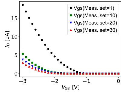
Fig. 4: Measured I-V curves in the “Vgs” stress condition at  $V_{stress} = -4.0V$ . Both the x-intercept and the slope of the curves change as total stress period becomes longer. This observation suggests degradation models are necessary for both threshold voltage and carrier mobility shift.
