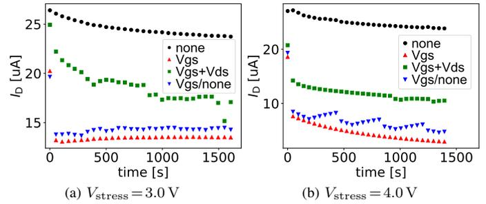
Fig. 5: Measured drain currents at  $V_{GS} = V_{DS} = -3.0V$ . Larger degradation has been observed in (b) than that in (a). The trend of current recovery is clearer in the alternative stress condition (Vgs/none).
