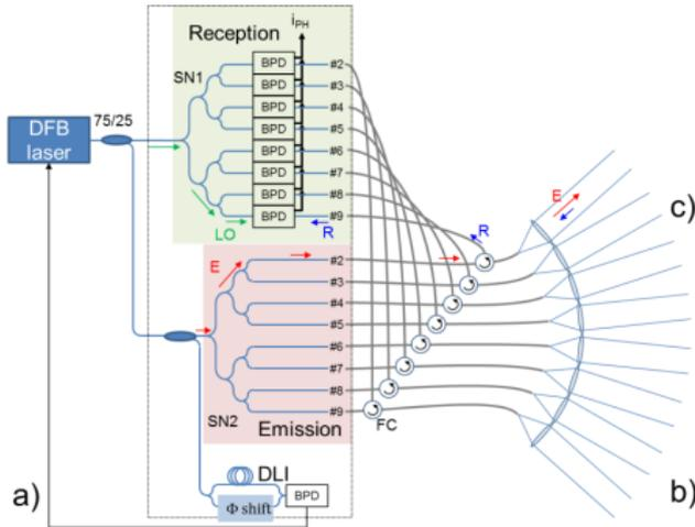
Fig. 2. Architecture of the FMCW Lidar system (the rectangle delimits the chip perimeter).
