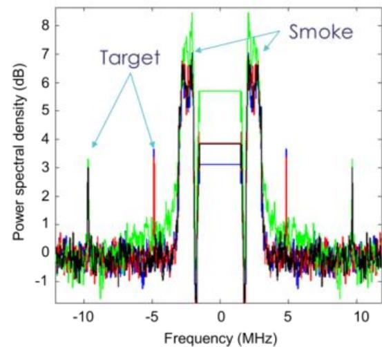
Fig. 1. Experimental power spectral density of a target behind a cloud.
