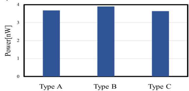
Fig.5 Comparison of TE power of three types of  $\mu$ -TEG.
