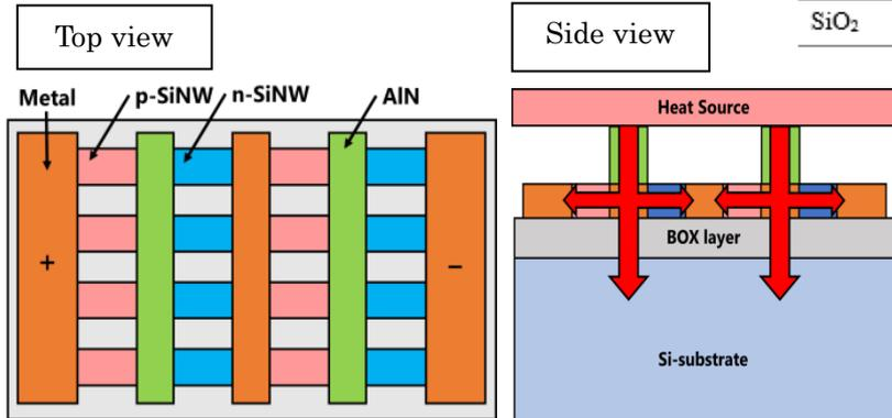
Fig 1 Schematic of the cavity-free  $\mu$ -TEG.
