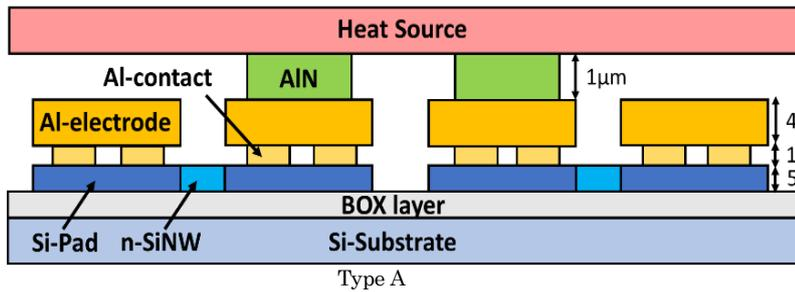
Fig 3 Cross-sectional view of 3 types  $\mu$ -TEG structure.
