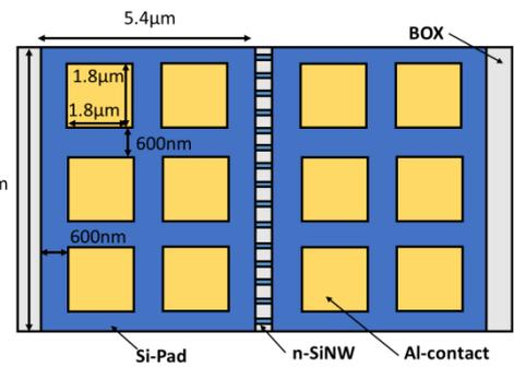
Fig2. Top view of SOI and Al-contact layer
