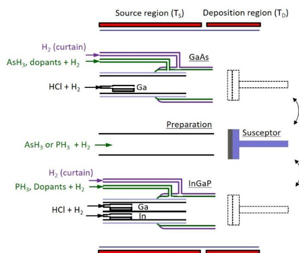
Fig. 1 The schematic of growth chambers of the custom-built quartz HVPE reactor utilized.
