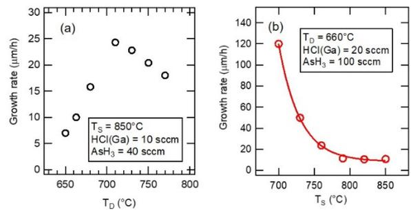
Fig. 2 The growth rate of GaAs as a function of (a)  $T_D$  and (b)  $T_S$ .
