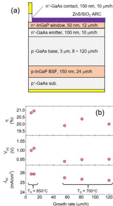
Fig. 3 (a) Schematic structure of GaAs solar cells used and (b) cell performance of GaAs solar cells as a function of the growth rate.
