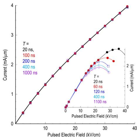
Fig. 2 Main panel plots the results of pulsed current–voltage measurements of an h-BN-encapsulated monolayer graphene FET. Results are shown for various pulse durations ( $T$ , indicated), and the solid line is a guide to the eye. Inset: corresponding measurements for a (bilayer) graphene-on-SiO<sub>2</sub> device. Figure from Ref. 3. Copyright 2019 American Chemical Society.
