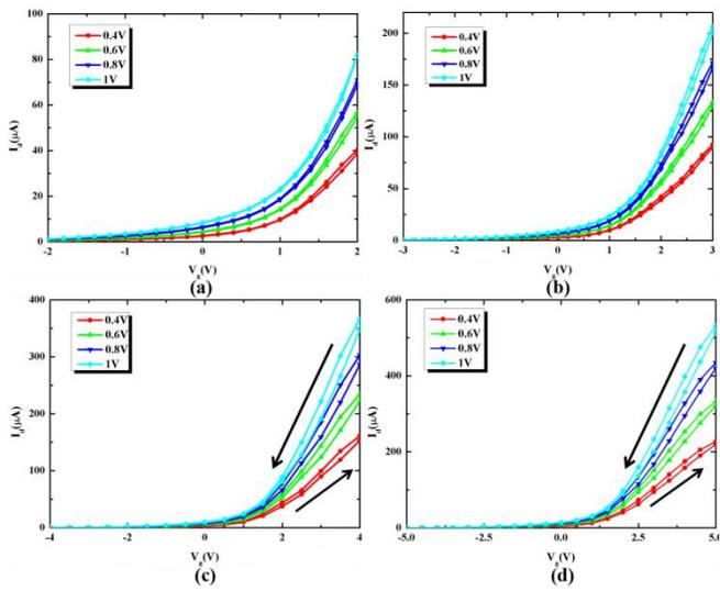
Fig. 3 Transfer curves of the HZO/MoS<sub>2</sub> FeFET at increasing  $V_g$  range with linear y-axis.
