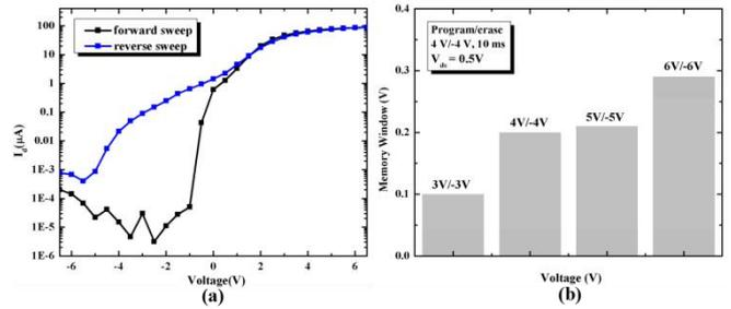
Fig. 4 (a) Transfer curves of the HZO/MoS<sub>2</sub> FeFET with the logarithmic y-axis. (b) Extracted MWs under different program/erase (P/E) conditions.
