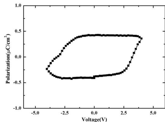
Fig. 2 P-V curve of a Au/HZO/p+ Si MIS capacitors.
