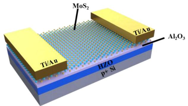
Fig. 1 3D schematic image of the MoS<sub>2</sub> back-gate transistor with ferroelectric HZO gate dielectrics.
