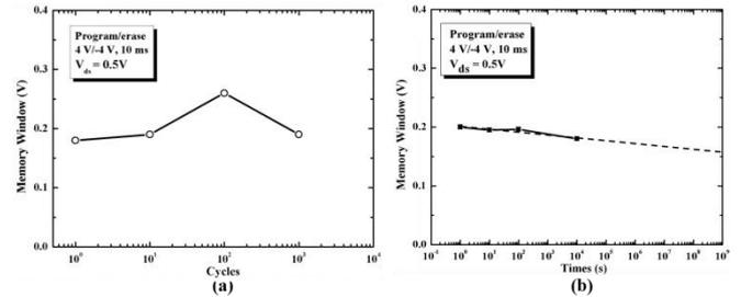
Fig. 5 (a) Endurance measurements under P/E pulse conditions. (b) Retention characteristic of the HZO/MoS<sub>2</sub> FeFET.
