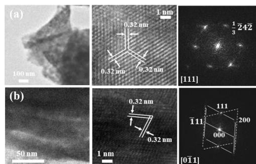
Fig. 4(a) TEM, HRTEM, and FFT pattern of exfoliated nanosheets (plan view), (b) cross-sectional view.
