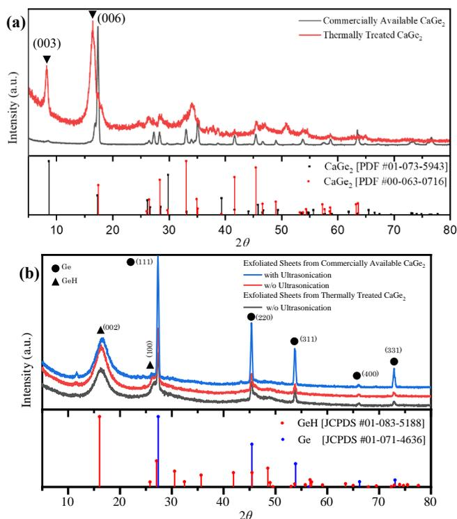
Fig. 1(a) XRD pattern for thermally-treated and commercially-available CaGe<sub>2</sub> (b) XRD pattern for exfoliated Ge-based nanosheets.
