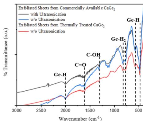
Fig. 2 FT-IR spectra of exfoliated Ge-based nanosheets with Ge-H stretching and wagging, weak vibrational modes of Ge-H<sub>2</sub>.
