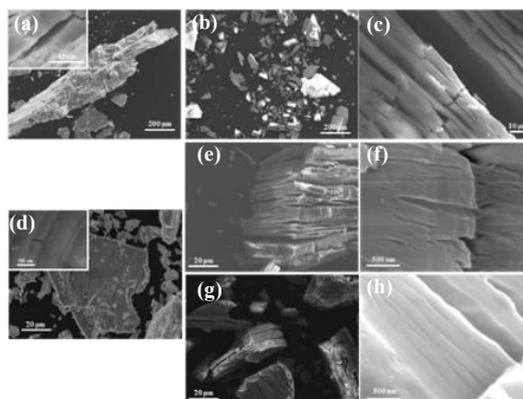
Fig. 3(a) FE-SEM images of thermally treated CaGe<sub>2</sub> (b)(c) exfoliated Ge-nanosheets w/o ultrasonication (d) commercially-available CaGe<sub>2</sub> and exfoliated Ge-nanosheets (e) (f) w/o ultrasonication (g)(h) with ultrasonication
