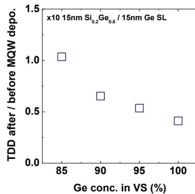
Fig. 4. Ratio between TDD before and after 10 cycles of  $\text{Si}_{0.2}\text{Ge}_{0.8}/\text{Ge}$  superlattice deposited on Ge or SiGe VS of various Ge concentrations. Thicknesses of SiGe layers and Ge layers of SL are 15 nm.
