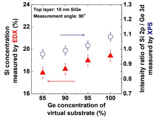
Fig. 3. Si concentration measured by EDX and intensity ratio of Si2p and Ge3d in SiGe / Ge superlattice grown on Ge or SiGe virtual substrate with different Ge content. Thickness of SiGe and Ge layers are 15 nm and top layer of the SiGe MQW is SiGe.
