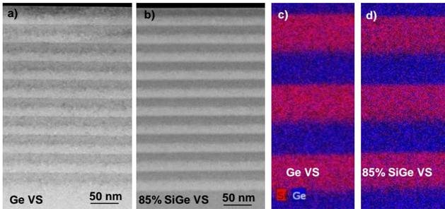
Fig. 1. a) Cross section bright field STEM images of 10 cycles of SiGe/Ge MQW deposited on a) Ge VS and b)  $\text{Si}_{0.15}\text{Ge}_{0.85}$ . c) and d) show Si and Ge distribution EDX mapping of the SiGe/Ge MQW on Ge VS and  $\text{Si}_{0.15}\text{Ge}_{0.85}$  VS, respectively
