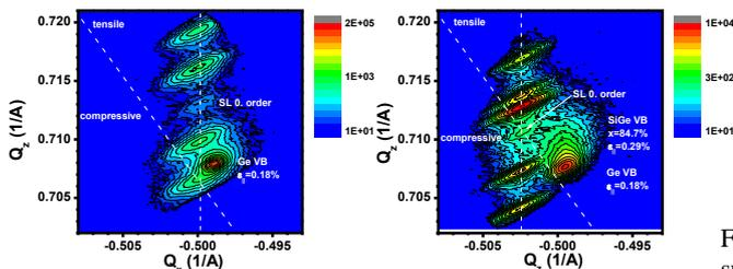
Fig. 2. XRD RSM images of 10 cycles of SiGe/Ge MQW deposited on a) Ge VS and b)  $\text{Si}_{0.15}\text{Ge}_{0.85}$ .
