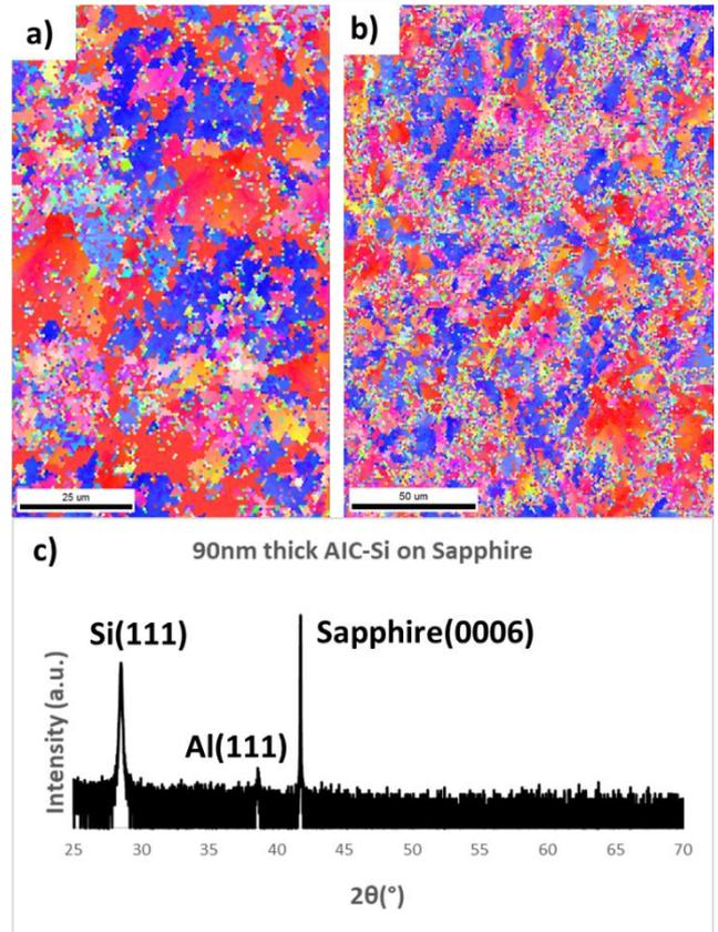
**Fig. 3** - Substrate effects on thicker Si films. EBSD of  $\sim 100$ nm AIC-Si on a) STO(001) b) glass showing a loss of preferential orientation with increasing thickness. c) XRD of thicker AIC-Si on sapphire showing that preferential Si(111) orientation is preserved. Note the Al peak is present because Al was not etched from the film surface.
