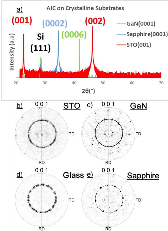
**Fig. 1** - Si(111) fabricated on crystalline substrates by aluminum-induced crystallization. a) XRD showing Si(111) formed on different crystalline substrates. b-e) EBSD pole figures showing the extent of orientation or misorientation relative to the  $\langle 111 \rangle$  for the AIC-Si films
