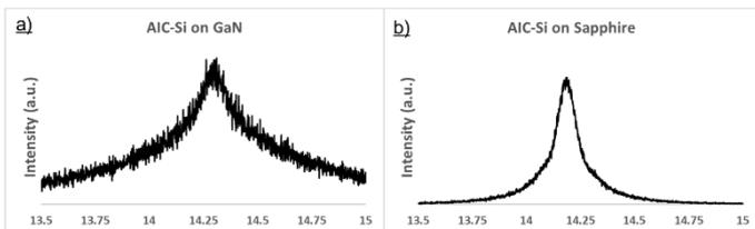
**Fig. 2** - X-ray rocking curves of AIC-Si on a) GaN and b) sapphire showing narrow full-width half-maximums.
