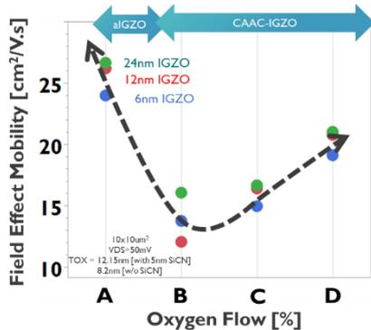
Fig. 6 Field effect mobility of a-IGZO and c-IGZO
