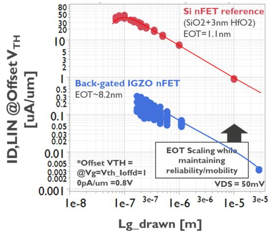
Fig. 8 Comparison of Back-gated IGZO nFETs with Si nFET reference
