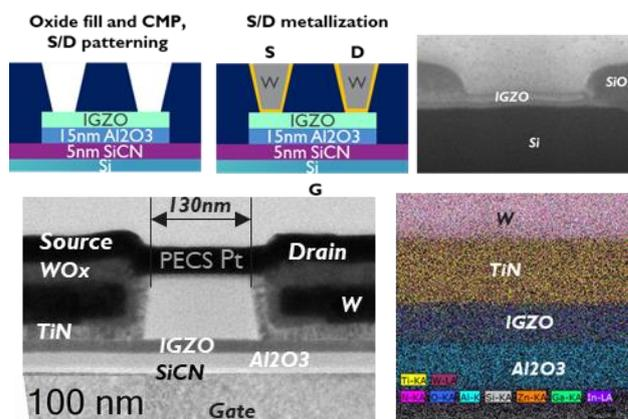
Fig. 2 Schematic cartoon of contact formation for Back-gated IGZO nFET, SEM after contact patterning, and TEM of the final device with  $L_g$  of 130nm with EDS map of IGZO under the contacts.
