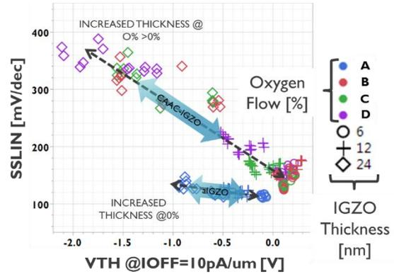
Fig 7. Electrostatics for a-IGZO and c-IGZO
