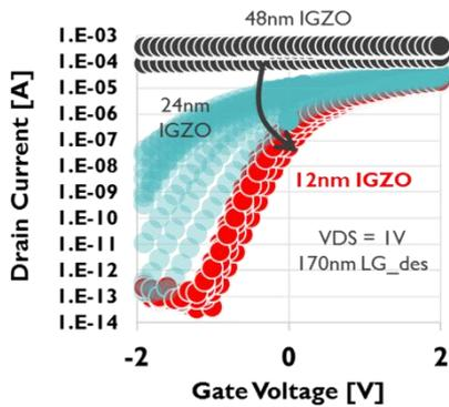
Fig. 5 Impact of a-IGZO thickness scaling on  $V_{th}$  swing
