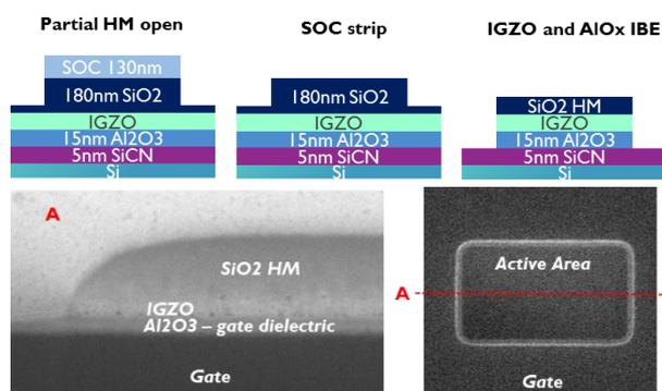
Fig. 1 Schematic cartoon of IGZO Active area formation and Top Down (TD) SEM of the Active Area.
