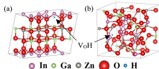
Fig. 1 (a) c-IGZO model and (b) a-IGZO model, which contained  $V_OH$  and were used for calculations.
