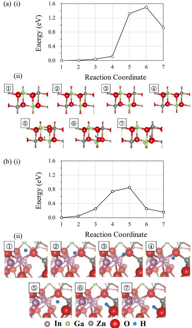
Fig. 3 (i) Total energies and (ii) atomic structures on minimum energy path of release of H from  $V_O$  calculated by NEB method in (a) c-IGZO model and (b) a-IGZO model. For clarity, structure images in (b)(ii) are enlarged.
