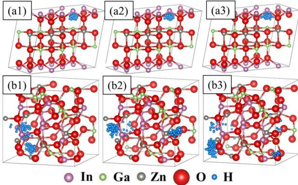
Fig. 2 Trajectories of H in FPMD simulations on c-IGZO model at (a1) 600°C, (a2) 800°C, and (a3) 1000°C, and on a-IGZO model at (b1) 600°C, (b2) 800°C, and (b3) 1000°C. Initial models contained  $V_OH$ . Although atoms other than H also moved, only initial atomic arrangement of them is shown here.
