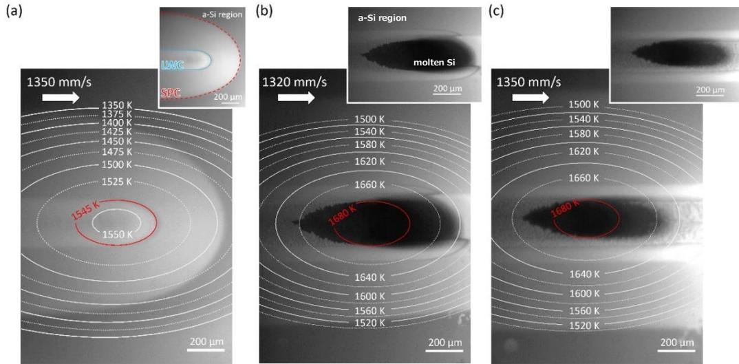
Fig. 2 Two-dimensional temperature distribution in the molten silicon region (a) during first irradiation on the a-Si films, (b) during second irradiation on the first crystallization and (c) during the third irradiation on the second crystallization (HSLC region). (intervals between dotted line and solid line: (a) 25 K, (b–c) 20 K) Inset images show the crystallization region and molten silicon region.
