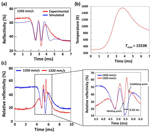
Fig. 3 (a) Relative reflectivity of the simulated result (blue line) and the experimental result (red line) during SPC crystallization. (b) Time-variation of temperature in Fig. 2(a). (c) Relative reflectivity with the scanning speed of 1350 mm/s (blue line) and 1320 mm/s (red line) during TPJ irradiation.
