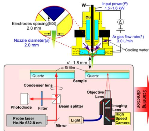
Fig. 1 Schematic illustration of the simultaneous measurement systems for obtaining the temperature distribution in molten silicon region.
