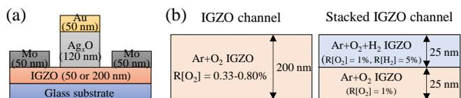
Fig. 1 (a) Schematic cross-sectional view of the IGZO MES-FET and (b) Two types of IGZO channels used in the experiments.
