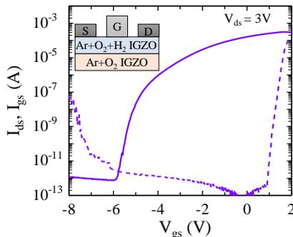
Fig. 4 Transfer characteristic of the MES-FET with an Ar+O<sub>2</sub>- and Ar+O<sub>2</sub>+H<sub>2</sub>-sputtered stacked IGZO channel.
