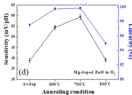
Fig. 2(a)-(d) Cyclic voltammograms of Mg-doped ZnO films (a) as-deposited and (b) annealed at 700 °C when immersed in solution with pH values from 2 to 12. Sensitivity and linearity of EIS devices with (c) pure ZnO and (d) Mg-doped ZnO as a function of RTA temperatures.
