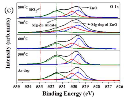
Fig. 4(c) XPS O 1s results of Mg-doped ZnO film with rapid thermal annealing.
