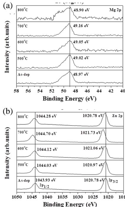
Fig. 4(a)-(b) XPS Zn 2p and Mg 2p results of Mg-doped ZnO film with rapid thermal annealing.
