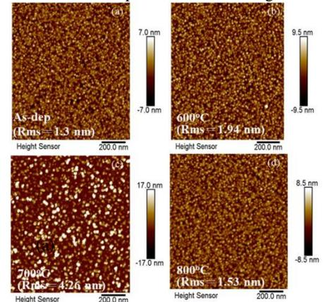
Fig. 5(a)-(b) (a) As-dep R<sub>rms</sub>=1.3(nm), (b) RTA at 700 °C R<sub>rms</sub>=4.26(nm)
