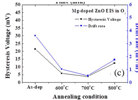
Fig. 3(c) Shows the samples with rapid thermal annealing at various conditions of hysteresis and drift rate.
