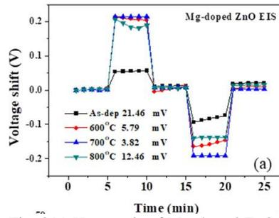
Fig. 3(a) Hysteresis of Mg-doped ZnO films during the pH loop of 7 → 4 → 7 → 10 → 7 over a period of 25 minutes.
