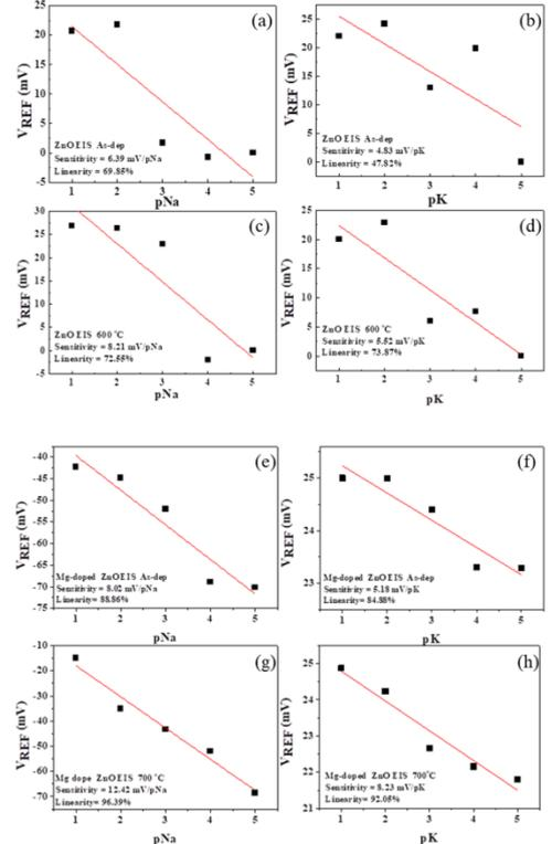
Fig. 6 Sensitivity and linearity of ZnO and Mg-doped ZnO sensing membranes toward sodium and potassium ions.
