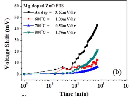
Fig. 3(b) Drift voltage of Mg-doped ZnO films dipped in pH 7 buffer solution for 12 hours.
