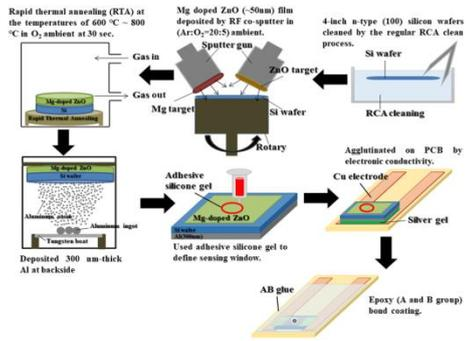
Fig. 1 Schematic of the fabrication process of Mg-doped ZnO sensing membrane.
