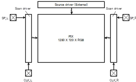
Figure 3 Display prototype configuration.
