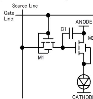
Figure 1 Subpixel circuit diagram.
