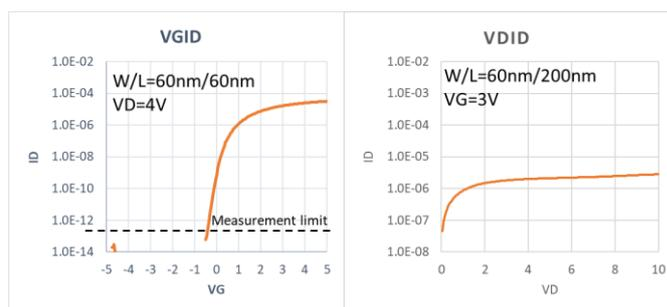
Figure 2 Performance of  $W/L = 60 \text{ nm}/60 \text{ nm}$  and  $W/L = 60 \text{ nm}/200 \text{ nm}$  CAAC-IGZO FET.
