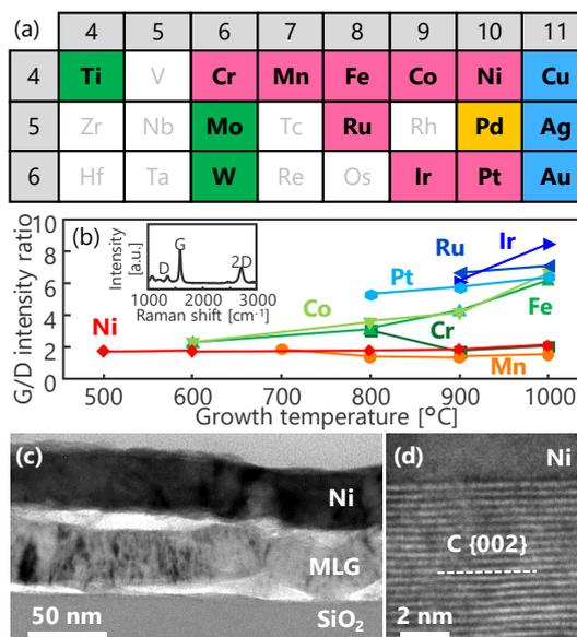
Fig. 2. (a) Periodic Table colored by the classification of interactions between metals and carbon. (b) G/D intensity ratio as a function of growth temperature in group (1). (c) Cross-sectional TEM image and (d) high-resolution lattice image of the Ni sample at 600 °C.
