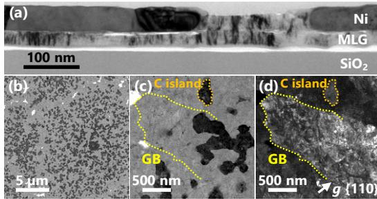
Fig. 4. Characterization of the sample for  $t = 50$  nm and  $t_{\text{AlO}_x} = 1$  nm. (a) Bright-field cross-sectional TEM image of as-annealed sample. Plane TEM image of the sample after Ni removal. Bright-field at (b) low and (c) high magnifications and (d) dark-field, showing the same area as (c).
