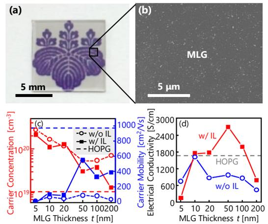
Fig. 5. (a) Photograph and (b) SEM image of the sample for  $t = 5$  nm without IL after Ni removal. Electrical properties of the MLG layers after Ni removal as a function of  $t$ . (c) Carrier concentration and (d) Carrier mobility. (d) Electrical conductivity.
