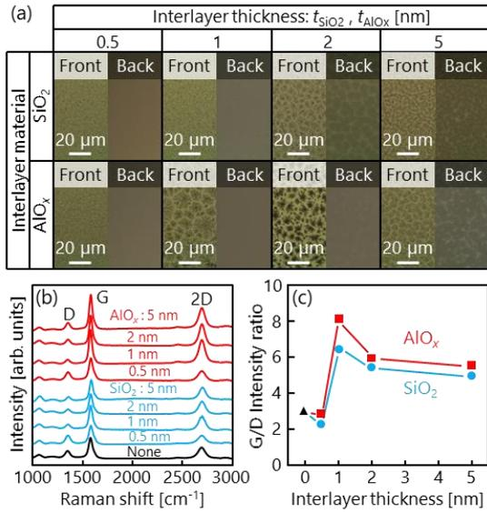
Fig. 3. Characterization of the sample for  $t = 50$  nm and  $t_{\text{AlO}_x} = t_{\text{SiO}_2} = 0-5$  nm. (a) Nomarski optical micrographs of the as-annealed samples. (b) Raman spectra obtained from the back side of the samples. (c) The G/D intensity ratio of the samples.
