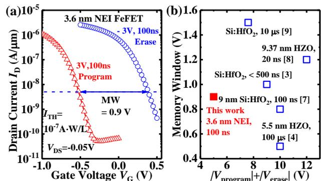
Fig. 2. (a)  $I_D-V_G$  characteristics from a 3.6 nm NEI FeFET for the two polarization states with 100 ns program/erase pulses. (b) Benchmarking of NEI FeFET memory with reported HfO<sub>2</sub>-based FeFETs on to MW and  $V_{\text{program}}+|V_{\text{erase}}|$ . NEI FeFET achieves low operating voltages while maintaining decent MW.
