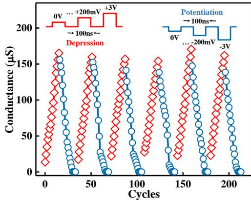
Fig. 4 Continuous modulations of conductance upon the repeated and alternated application of pulses. Insert shows the pulse shape of potentiation: 0V~+3V, depression: 0V~-3V.
