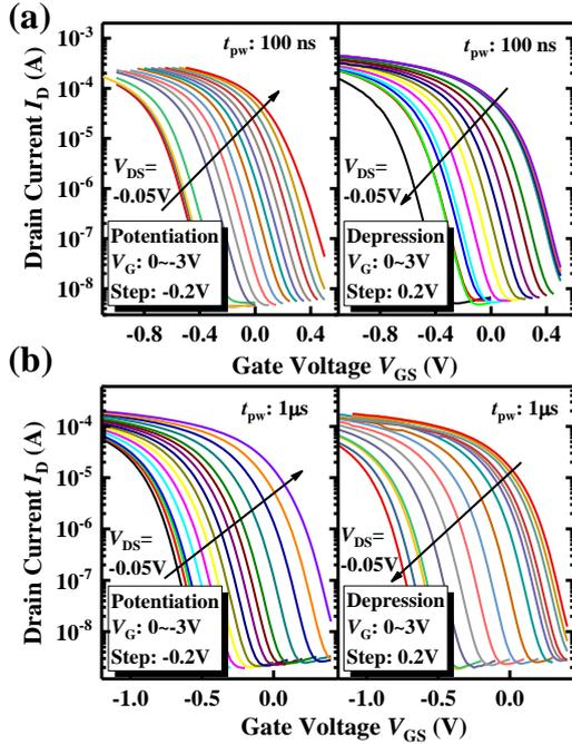
Fig. 3 NEI FeFET synapse behaviors: gradual tuning of  $I_D - V_G$  curves under (a) 100 ns and (b) 1  $\mu$ s voltage pulses for potentiation and depression operations.
