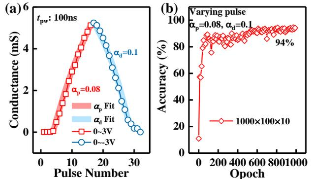
Fig. 5. (a) Demonstration of potentiation and depression of NEI FeFET synaptic weight (conductance) with varying-amplitude 100 ns voltage pulse trains. (b) Simulated CNN's learning accuracy evolution based on NEI FeFET synaptic behavior. 94% accuracy is achieved using varying-amplitude pulses.
