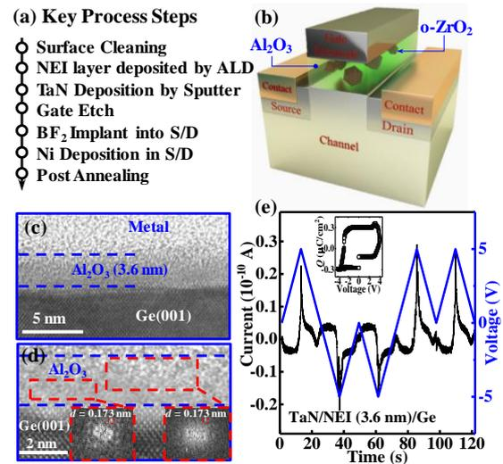
Fig. 1 (a) Key process steps for fabricating NEI FeFET. (b) 3D schematic of NEI FeFET. (c) XTEM images of the gate stack of FeFET with 3.6 nm NEI layer. (d) HRTEM image showing nanocrystals embedded in amorphous Al<sub>2</sub>O<sub>3</sub> for the sample. (e) PUND test of TaN/NEI(3.6 nm)/Ge capacitor, and the insert is the extracted  $Q-V$  loop.
