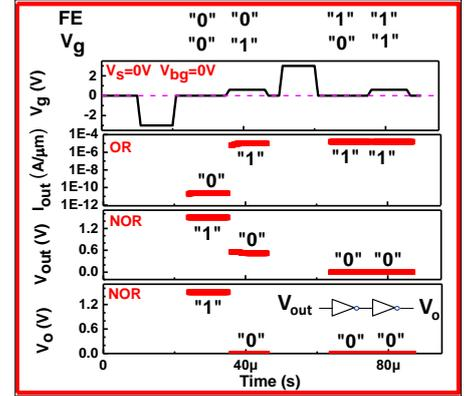
Fig. 5. Transient waveform for successfully realizing OR/NOR logic functionality for FeFET with  $V_s = V_{bg} = 0V$ .
