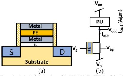
Fig. 1. (a) Schematic of MFMIS FeFET. (b) 1T FeFET based logic-in-memory circuit by connecting single FeFET with a pull-up (PU) resistor in series. Supply voltage  $V_{dd} = 1.5V$ . The resistance of PU is 100 k $\Omega$ .
