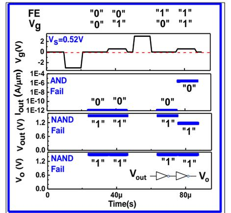
Fig. 8. Transient waveform of AND/NAND logic function for FeFET with large  $V_s$  ( $= 0.52V$ , larger than maximum  $V_s$  shown in Table I). FeFET with too large  $V_s$  fail to present the correct logic functionality.
