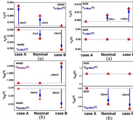
Fig. 10. Impact of FE parameter variations on the design space of (a)  $V_s$  and (b)  $V_{bg}$  for NAND logic gate. ( $V_{s,Max} - V_{s,Min}$ ) and ( $V_{bg,Max} - V_{bg,Min}$ ) are the design window for correct logic function.
