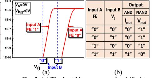
Fig. 3. (a) The  $I_{out}$ - $V_g$  curves can be shifted to the right by applying positive  $V_s$  or negative  $V_{bg}$ . (b) Truth table of AND/NAND logic gate.
