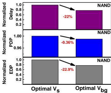
Fig. 9. Propagation delay, power-delay product (PDP), and energy-delay product (EDP) comparisons between NAND logic gate with optimal  $V_s$  and  $V_{bg}$  designs.
