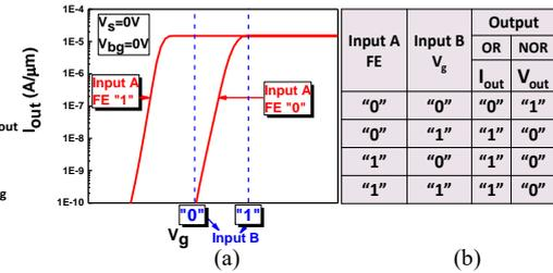
Fig. 2. (a) Schematic illustration of OR/NOR logic gate for FeFET shown in Fig. 1(b) with  $V_s = V_{bg} = 0V$ . By applying adequate  $V_g$  pulse, the FE polarization can be switch between "0" and "1" states. (b) Truth table of OR/NOR logic functionality. FE polarization state and  $V_g$  are the two input of OR/NOR logic gate.
