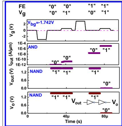
Fig. 7. Transient waveform of correct AND/NAND logic function for FeFET with optimal  $V_{bg}$  design ( $= -1.742V$ ).
