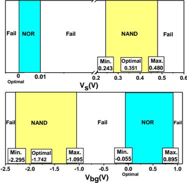
Fig. 4. Design space of  $V_s$  (up) and  $V_{bg}$  (bottom) for successful NAND/NOR logic functionality.  $V_s$  and  $V_{bg}$  applied to FeFET within the design window result in correct logic functionality.
