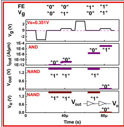
Fig. 6. Transient waveform of correct AND/NAND logic function for FeFET with optimal  $V_s$  design ( $= 0.351V$ ).
