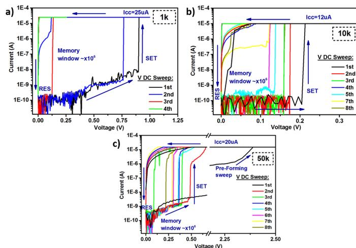
Fig. 2 – Threshold switching (TS) behavior of the Ag/N-GOQDs/Pt devices with a) 1k deposited N-GOQDs thin film, b) 10k deposited N-GOQDs film, and c) 50k deposited N-GOQDs film
