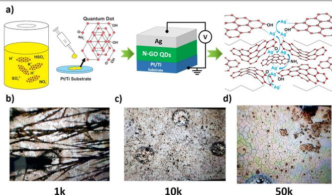
Fig. 1 – a) Solution fabricated N-GOQDs and Ag/N-GOQDs/Pt device with I-V set up, b) Optical microscopy (OM) image of 1k processed N-GOQDs thin film, c) 10k processed N-GOQDs film, and d) 50k processed N-GOQDs film.
