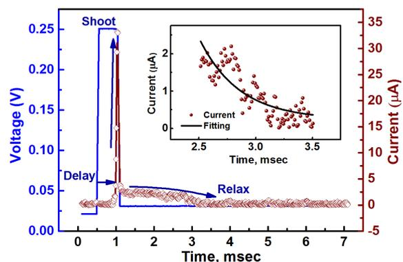
Fig. 3 – Shoot-Delay-Relax pulse characteristics of the Ag/N-GOQDs/Pt for the best TS performer 10k double coated thin film.
