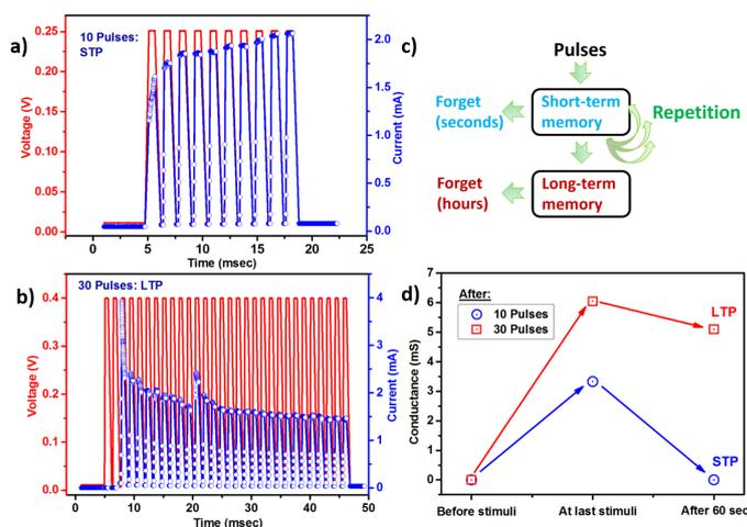
Fig. 4 – a) Short-term memory (STP; 10 Pulses) and b) Long-term memory (LTP; 30 Pulses) Pulse I-V characteristics of Ag/N-GOQDs/Pt best TS performer (10k) device and according c) Atkinson n' Shiffrin memorization model, and d) STP & LTP retention of the device after 10 and 30 stimuli, respectively.
