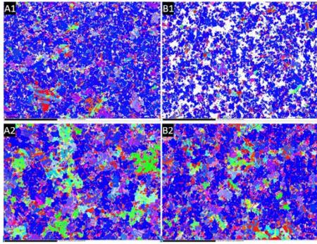
Fig. 1 Inverse pole figure maps (ND) of Cu films, A1: 550 nm with EA, B1: 550 nm with EB, A2: 1000 nm with EA, and B2: 1000 nm with EB. The scale bar is 20  $\mu\text{m}$ .
