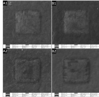
Fig. 3 HIM images of Cu films after the dose of  $7 \times 10^{17}$  ions  $\text{cm}^{-2}$  by HIM. The scale bar is 200 nm.
