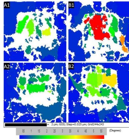
Fig. 4 Grain Orientation Spread (GOS) maps for each Cu film after the dose of  $7 \times 10^{17}$  ions  $\text{cm}^{-2}$  by HIM.
