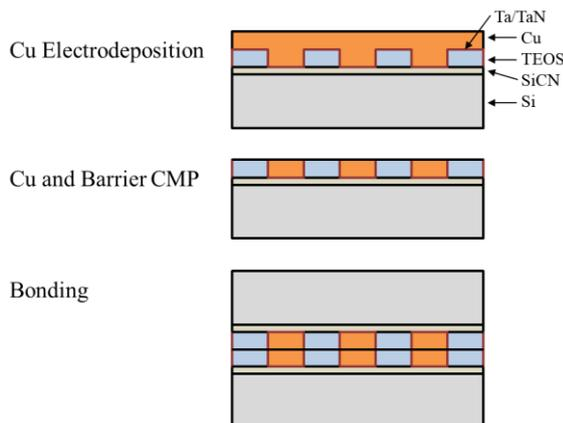
Fig. 3 Bonding Process Flow of Patterned Wafers.
