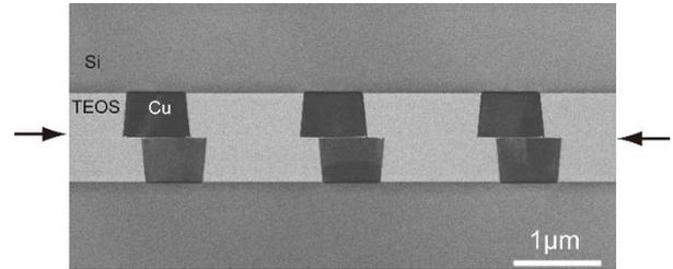
Fig. 5 TEM Micrograph of Bonded Wafers. [5]
