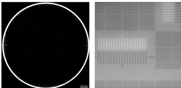
Fig. 4 Bonding Results of Patterned Wafers.
