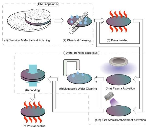
Fig. 1 Process flow of wafer bonding. [5]
