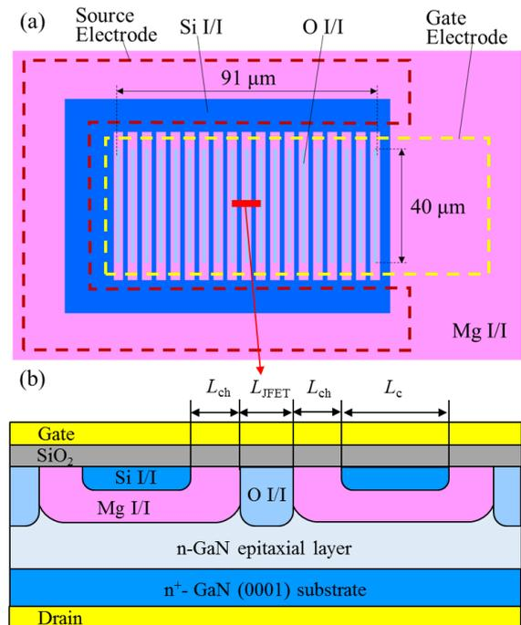
Fig. 1 Schematic images of vertical GaN planar MOSFETs with all ion implantation process. (a) plan view without SiO<sub>2</sub> layer, (b) cross sectional image of active region
