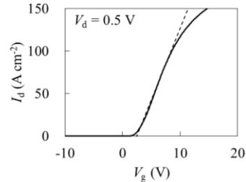
Fig. 3  $I_d$ - $V_g$  transfer characteristics of fabricated GaN MOSFET
