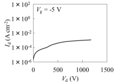
Fig. 4  $I_d$ - $V_d$  breakdown measurement of fabricated GaN MOSFET
