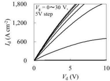
Fig. 2  $I_d$ - $V_d$  output characteristics of fabricated GaN MOSFET
