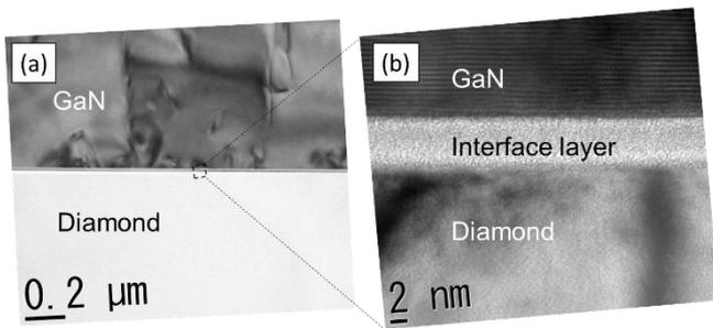
Fig. 2 Cross-sectional TEM images of a fabricated GoD HEMT observed with (a) a wider range and (b) a narrower range.
