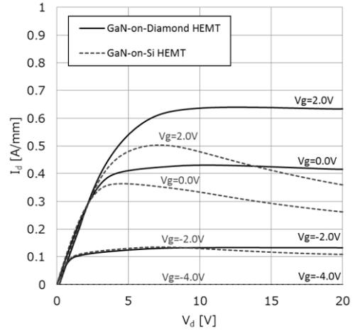
Fig. 3 Measured  $I_d$ - $V_d$  characteristics of GoD HEMT (solid lines) and GoSi HEMT (dashed lines).
