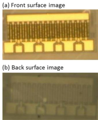
Fig. 1 Photographs of a fabricated GoD HEMT taken from (a) a front side of the HEMT and (b) a back side of the diamond substrate.
