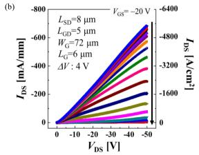
Fig.3  $I_{DS}$ - $V_{DS}$  characteristics. (a) The maximum drain current density was -250 mA/mm at  $V_{DS}$  and  $V_{GS}$  of -20 V and -20 V. (b) The maximum drain current density was -680 mA/mm at  $V_{DS}$  and  $V_{GS}$  of -50 V and -20 V. ( $W_G$  = 72 µm,  $L_{SD}$  = 8 µm,  $L_{GD}$  = 5 µm)
