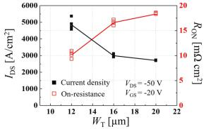
Fig.5 The hexagonal trench side ( $W_T$ ) dependence of drain current density at  $V_{DS}$  of -50 V and  $V_{GS}$  of -20 V, and specific on-resistance. Drain current density are indicated by closed symbol and specific on-resistance are indicated by opened symbol.
