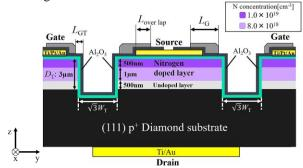
Fig.1 Cross sectional image of vertical-type diamond MOSFETs.
