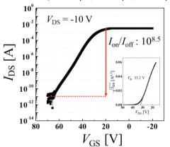
Fig.4  $I_{DS}$ - $V_{GS}$  characteristics at room temperature. On/off ratio was 8.5 orders of magnitude. Threshold voltage is 33.2 V.
