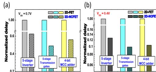
**Fig. 3.** Comparison of delay improvement in 5-stage inverter, transmission-gates and dynamic MCC adder using 2D-NCFETs. The transmission gates and MCC adder exhibit larger delay improvement than the inverter counterpart.
