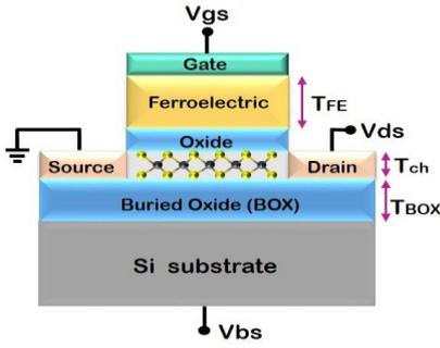
**Fig. 1.** Schematic of a MFIS-type 2D-NCFET (MoS<sub>2</sub>-n, WSe<sub>2</sub>-p) with channel thickness ( $T_{ch}$ ) = 0.65nm, EOT=0.65nm and BOX thickness ( $T_{BOX}$ )=5nm
