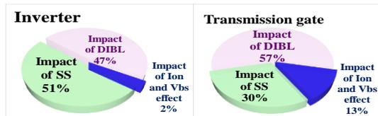
**Fig. 5.** Dissection of delay improvement for 5-stage inverter and transmission gate using 2D-NCFETs with (a)  $A_v=1.16$  and (b)  $A_v=1.72$
