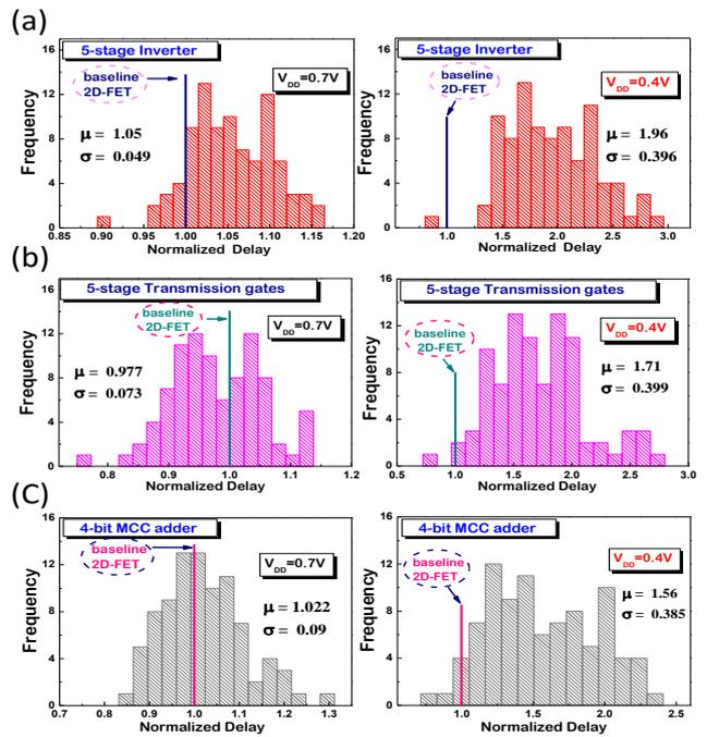
**Fig. 8.** Delay distributions for (a) 5-stage inverters (b) 5-stage transmission gates and (c) 4-bit MCC adder with 2D-NCFETs at  $V_{DD}=0.7V$  &  $0.4V$  using Monte-Carlo simulation. The mean value and sigma of delay are normalized to baseline 2D-FETs.
