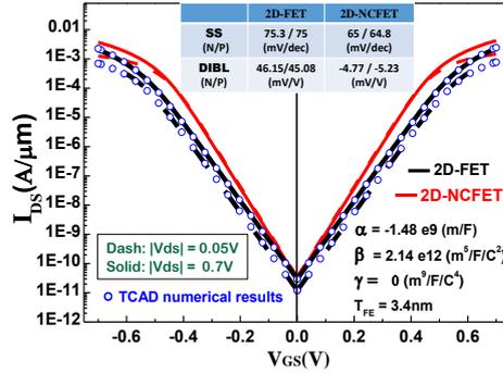
**Fig. 2.** Hysteresis-free  $I_{ds}$ - $V_{gs}$  characteristics of the simulated 2D-FETs and 2D-NCFETs with equal  $I_{OFF,Sat}$ . Reduced DIBL for the NCFET can be seen
