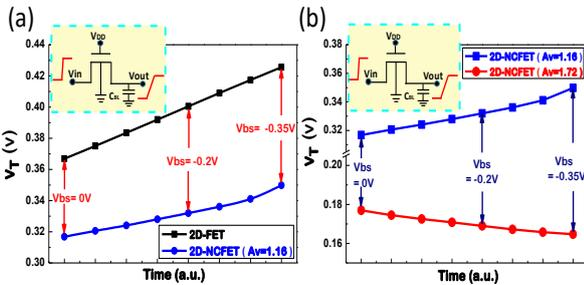
**Fig. 6.** Comparison of time dependence in  $V_T$  between (a) 2D-FET versus 2D-NCFET with  $A_v=1.16$  and (b) 2D-NCFET with  $A_v=1.16$  and 1.72 during switching in the NMOS pass gate.
