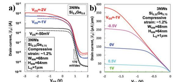
**Fig. 10:** a)  $I_D-V_G$  characteristics of the 3-stacked s-SiGe GAA pFETs.  $V_{th}$  does not shift positively with higher Ge %, indicative of high quality channels. b)  $I_D-V_{DS}$  characteristics. The drain current is normalized by the perimeter of NWs.
