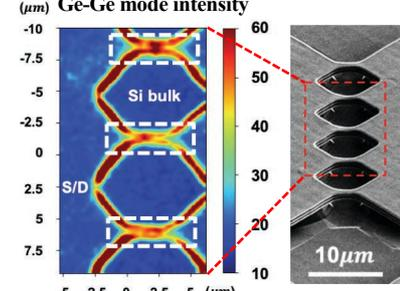
**Fig. 5:** Raman spectral imaging along with the corresponding SEM image. Ge enrichment takes place in the channel (white dotted box) whereas S/D remain Si-rich SiGe owing to Si sandwiched by SiGe.
