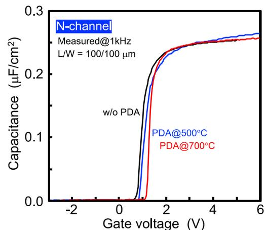
Fig. 3:  $C_{gc}-V_g$  curves of the n-channel MOSFETs for the various PDA conditions.
