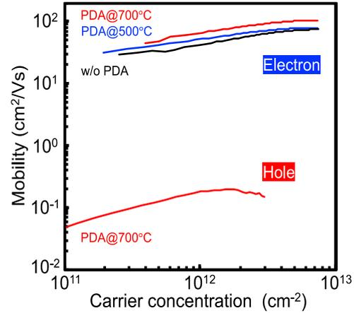
Fig. 7: Electron and hole mobilities as a function of the carrier concentration.
