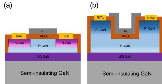
Fig. 2 : Schematic cross-sectional views of (a) n- and (b) p- channel GaN MOSFETs
