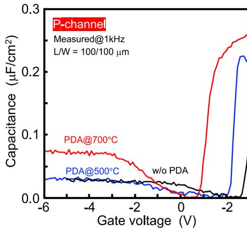
Fig. 5:  $C_{gc}$ - $V_g$  curves of the p-channel MOSFETs for the various PDA conditions.
