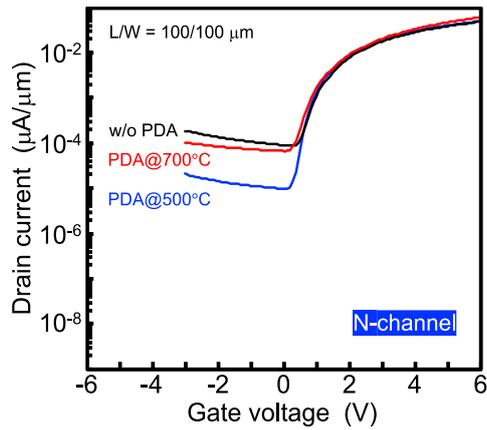
Fig. 4:  $I_d$ - $V_g$  curves of the n-channel MOSFETs for the various PDA conditions.
