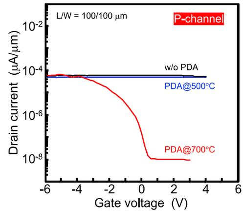
Fig. 6:  $I_d$ - $V_g$  curves of the p-channel MOSFETs for the various PDA conditions.
