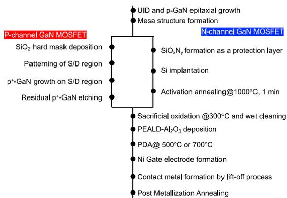
Fig. 1 : Fabrication process flows for the GaN MOSFETs
