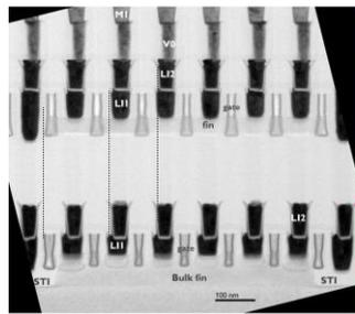
**Fig. 2.** TEM cross-section image of the fabricated 3D stacked finfets, along fins and across gates showing the tight alignment achieved by the top processed layers (Gate, Li1, Li2) toward the bottom layers.
