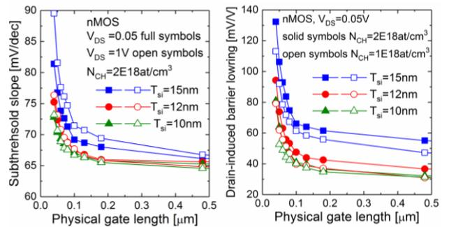
**Fig. 7** (a) SS and (b) DIBL vs.  $L_G$  of top tier planar NMOS devices in linear ( $V_{DS}=0.05V$ ) and saturation ( $V_{DS}=1V$ ) operation for different channel thickness (10,12,15nm) and different channel doping (1, 2, 3E18at/cm<sup>3</sup>)
