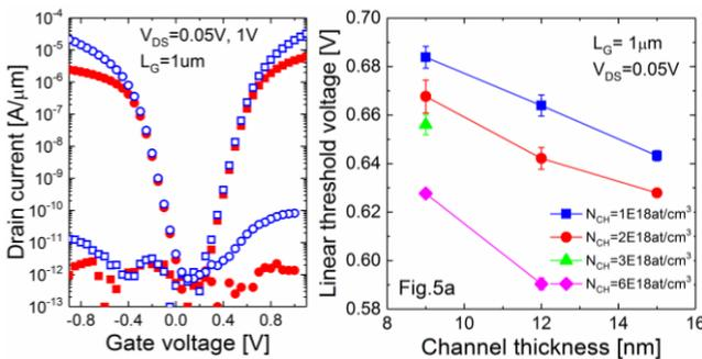
**Fig. 6** (a)  $I_D$ - $V_G$  of short channel top tier planar PMOS and NMOS devices in linear ( $V_{DS}=0.05V$ ) and saturation ( $V_{DS}=1V$ ) operation, (b) Threshold voltage dependence with channel thickness and channel doping in top tier NMOS devices.
