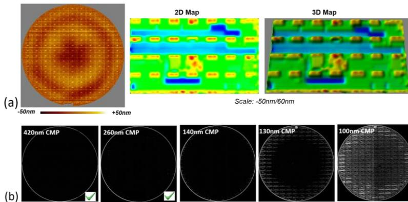
**Fig. 4** (a) Patterned wafer geometry (PWG) of carrier wafer after full processing. Map of the nano-topography peak to valley value on full wafer and 2D and 3D plots at die level (b) High resolution Scanning acoustic microscope (HR SAM) images after wafer to wafer bonding of a blanket donor wafer onto the patterned carrier wafer processed with different amounts of planarization of the bonding oxide.
