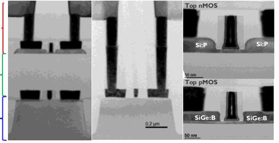
**Fig. 3.** TEM cross-section of the 3D stacked planar devices (a) stacked top and bottom tier devices with nanometric alignment, (b) 3D contacts to the bottom devices and (c) magnified top tier P and NMOS devices.
