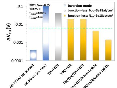
**Fig. 9** PBTI  $V_{TH}$  shifts at for junction-less top tier finfets with various gate stacks and reference inversion-mode devices with and without reliability anneal.
