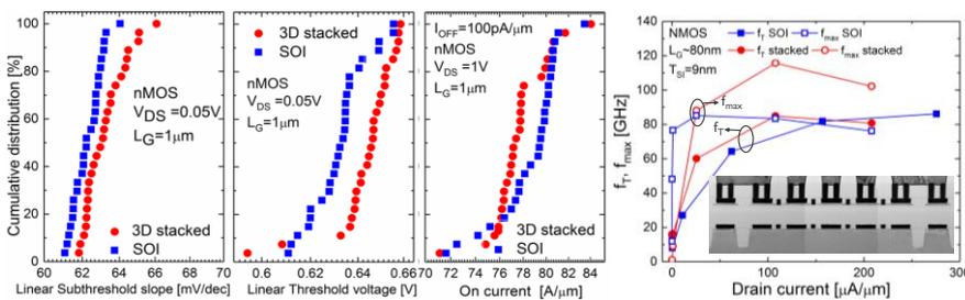
**Fig. 8** (a) Cumulative distribution of SS,  $V_T$ , and  $I_{ON}$  comparing junction-less 3D stacked finfets and SOI finfets (b)  $f_T$  and  $f_{max}$  comparing junction-less 3D stacked and SOI planar devices. Inset TEM cross-section of the RF structure.
