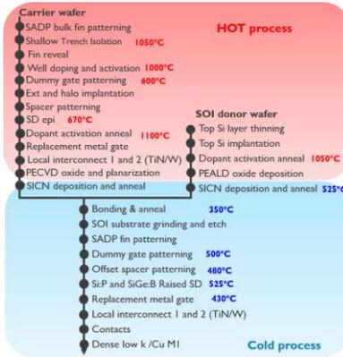
**Fig. 1.** Process flow of the 3D stacked finfets.
