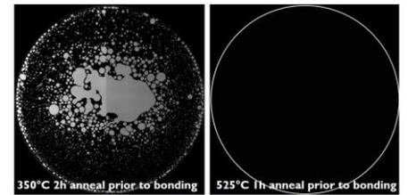
**Fig. 5** HR Scanning acoustic microscope image after wafer bonding of a donor wafer onto a bottom carrier wafer, and a post bonding anneal at 525°C for 1h (mimicking the top device thermal budget). Degassing anneal before bonding is: 350°C 2h (left) and 525°C 1h (right).
