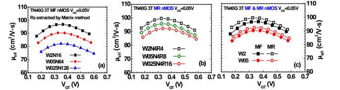
Fig. 7.  $\mu_{eff}$  vs.  $V_{GT}$  extracted from linear I-V characteristics (a) MF nMOS (b) MR nMOS (c) comparison of MF and MR nMOS with various  $W_F$  and  $N_F$
