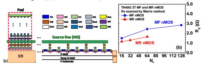
Fig. 3 (a) The cross section of MF device with the source line including contacts to S/D (b)  $R_S$  extracted by matrix method for MF and MR nMOS
