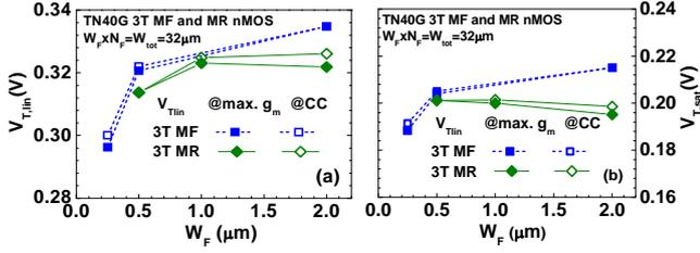
Fig. 4 Comparison of MF and MR nMOSFETs (a) linear region :  $V_{Tlin}$  vs.  $W_F$  at  $V_{DS} = 50$  mV (b) saturation region :  $V_{Tsat}$  vs.  $W_F$  at  $V_{DS} = 0.9$  V
