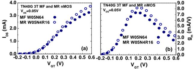
Fig. 6 Comparison of MF and MR nMOS : W05N64 and W05N4R16 (a)  $I_{DS}$  vs.  $V_{GT}$  (b)  $g_m$  vs.  $V_{GT}$  ( $V_{DS}=0.05$ V)
