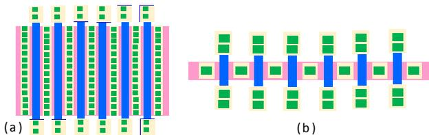
Fig. 1 Schematics of MF nMOS layouts with various  $W_F$  and  $N_F$  at fixed  $W_F \times N_F = 32\mu m$  (a) W2N16 (b) W025N128.
