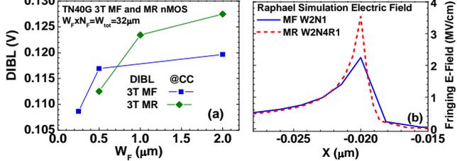
Fig. 5 Comparison of MF and MR nMOSFETs (a) DIBL versus  $W_F$  (b) finger-end fringing field along the channel direction and near the OD/STI corner region calculated by Raphael simulation.
