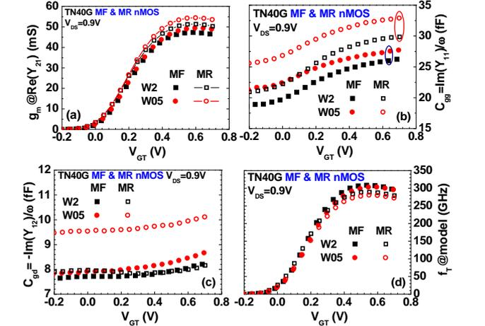
Fig.8 Comparison of MF and MR nMOS (a)  $g_m = \text{Re}(Y_{21})$  (b)  $C_{gg} = \text{Im}(Y_{11})/\omega$  (c)  $C_{gd} = -\text{Im}(Y_{12})/\omega$  and (d)  $f_T @ \text{model} = g_m / 2\pi(C_{gg} - C_{gd})^{1/2}$  vs.  $V_{GT}$  ( $V_{DS}=0.9$ V)
