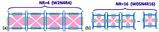
Fig.2 Schematics of MR nMOS layouts with various  $W_F$ ,  $N_F$ , and NR at fixed  $W_F \times N_F \times NR = 32\mu m$  (a) W2N4R4 (b) W05N4R16.
